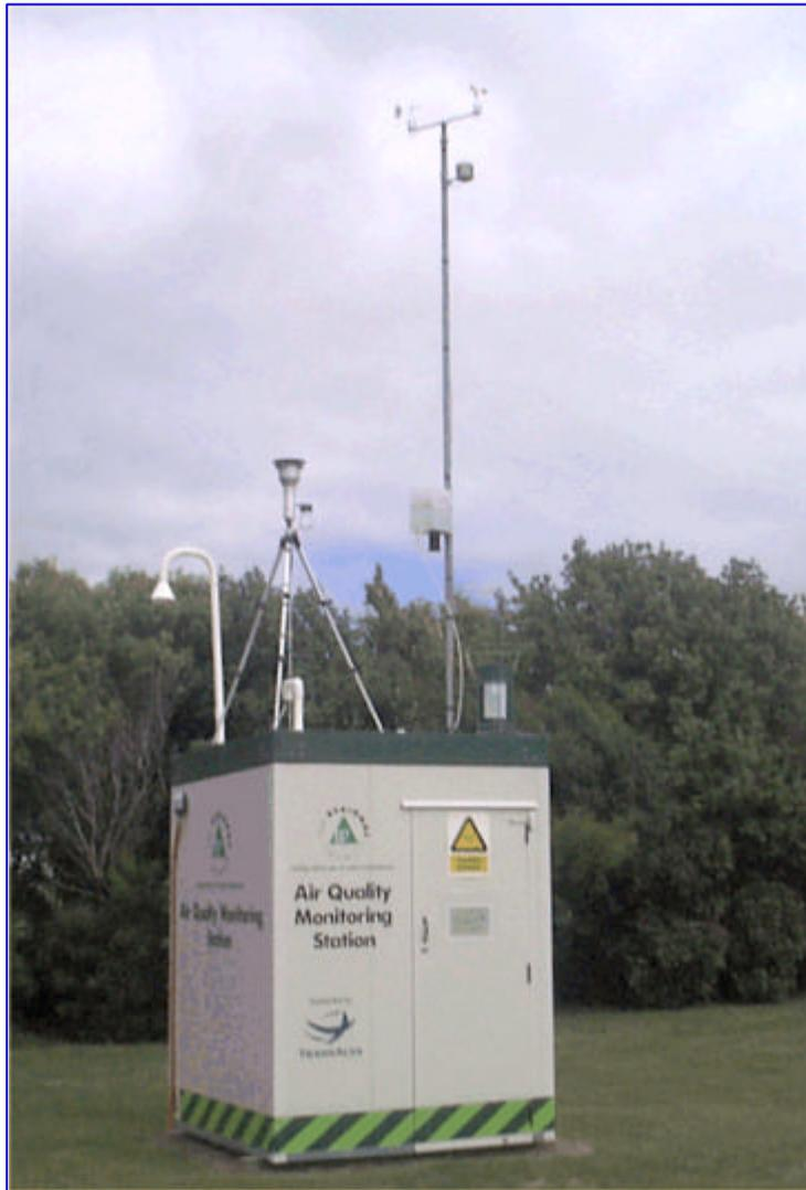
Figure 3.1 Mobile Air Quality Monitoring Station
