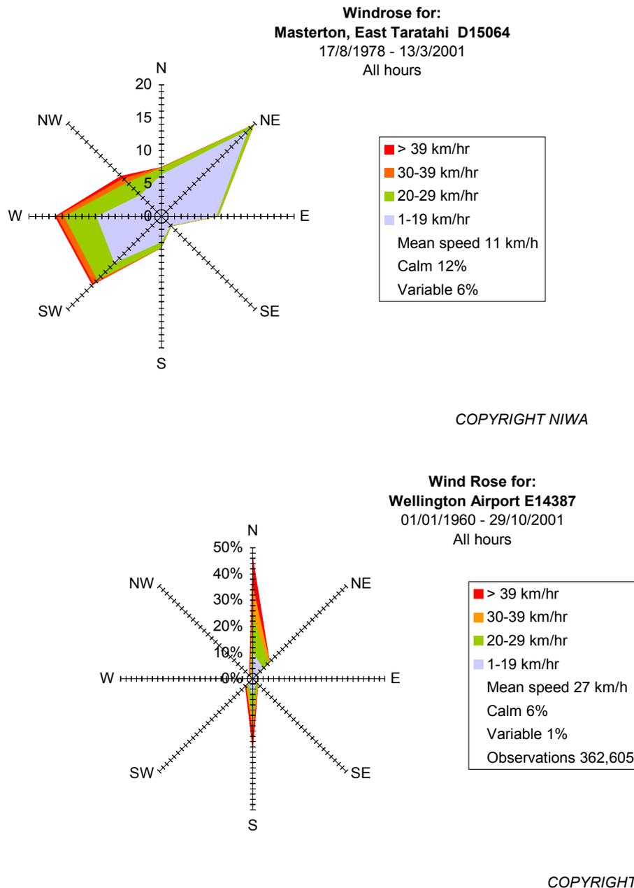
**Figure 1.3:** Wind roses for Masterton, East Taratahi and Wellington Airport. The scale on the axes represents the percent frequency and the colour depicts the mean speed for winds emanating from the direction indicated.
