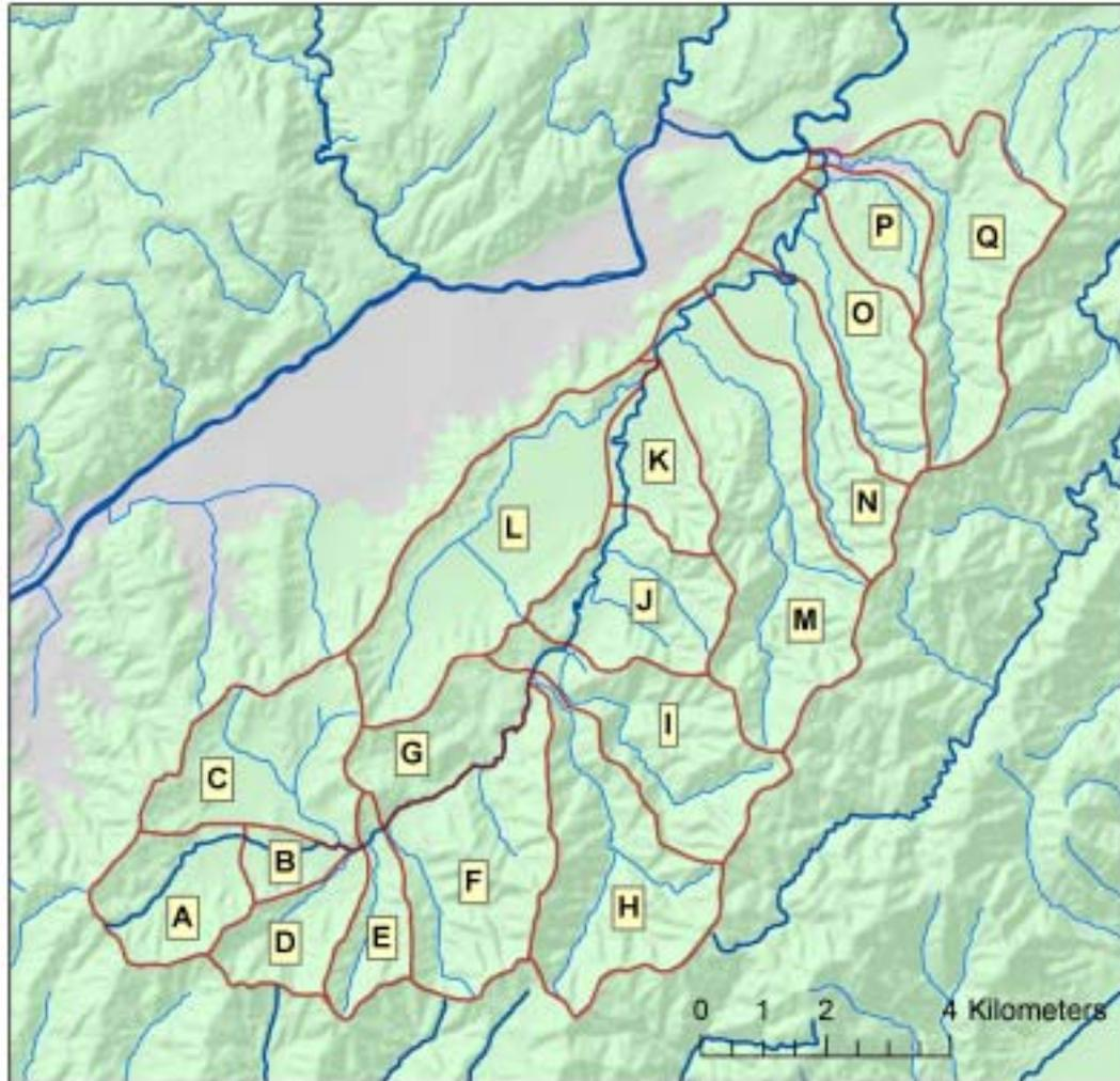
Figure 8: Schematic diagram of the rainfall runoff model of the Mangaroa catchment
