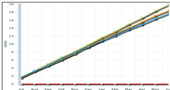
Kaiwharawhara Pump Station has used 16% less than last year. Some of this is due to reduced demand but is mostly due to the increased efficiency achieved from modifications to the pump wear rings.
