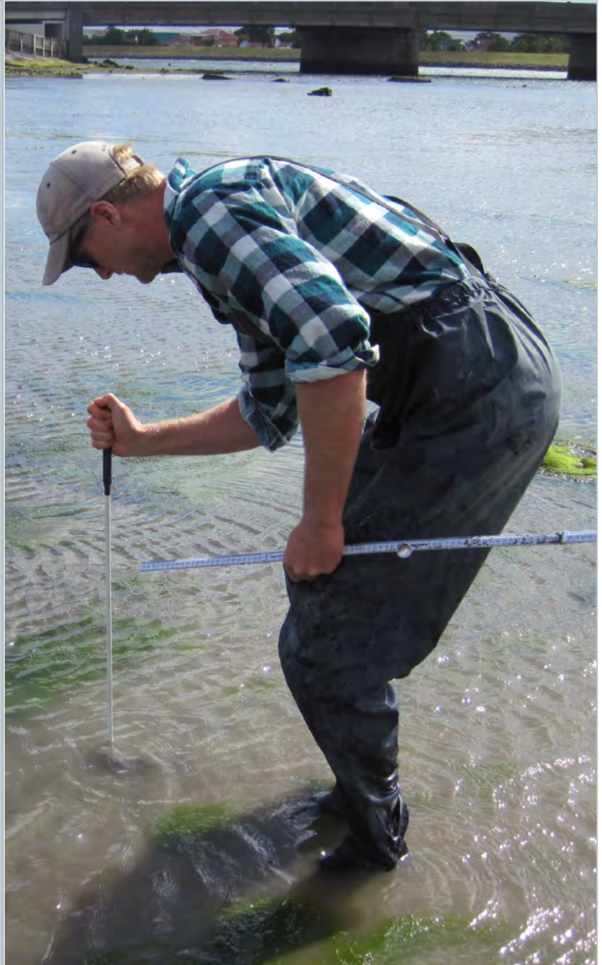
Measuring sediment plates in the lower Hutt Estuary, Jan 2015.
