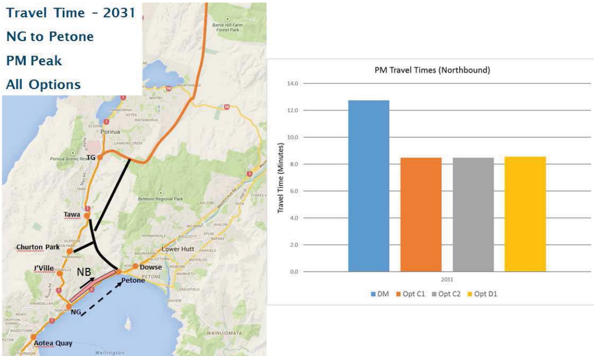
Figure 29 - Travel time between the Ngauranga Interchange and Petone Overhead Bridge 2031 Northbound PM Peak
