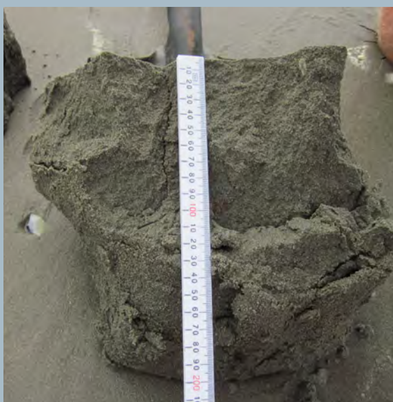
Representative vertical profile showing even colouring throughout, indicating well oxygenated sandy sediment.
