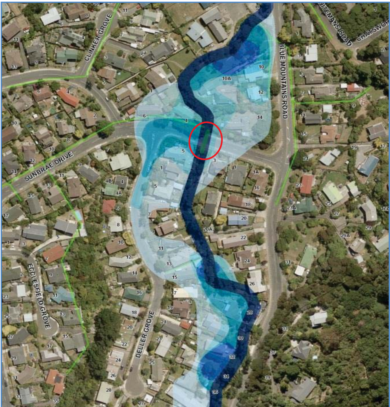
Figure 7 – Modelled flood depth at Sunbrae Drive
