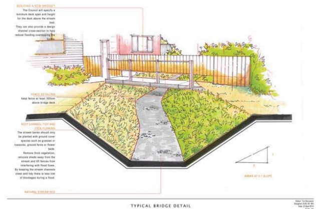
Figure18: Typical cross section of replacement bridge
