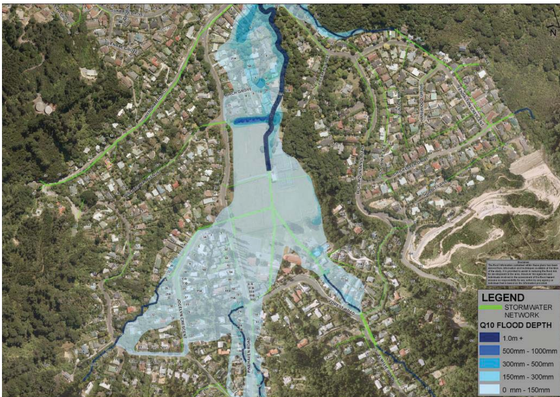
Figure 4.1 – Base scenario Q10 flood inundation
