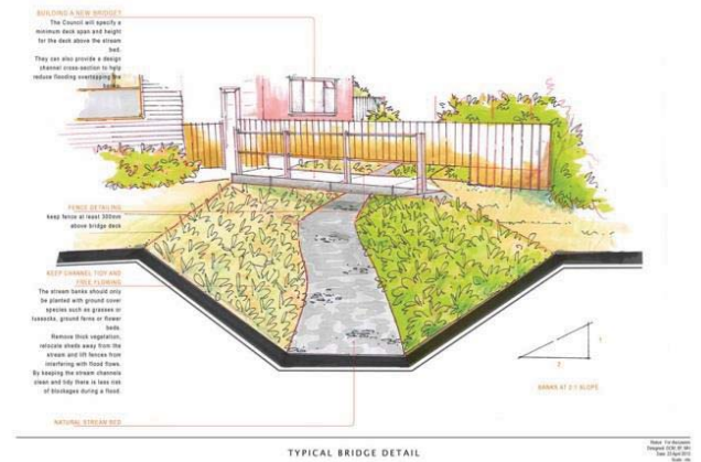
Figure18: Typical cross section of replacement bridge
