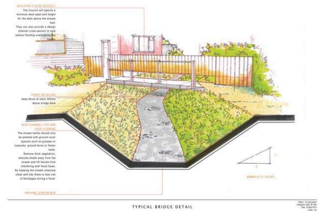
Figure18: Typical cross section of replacement bridge
