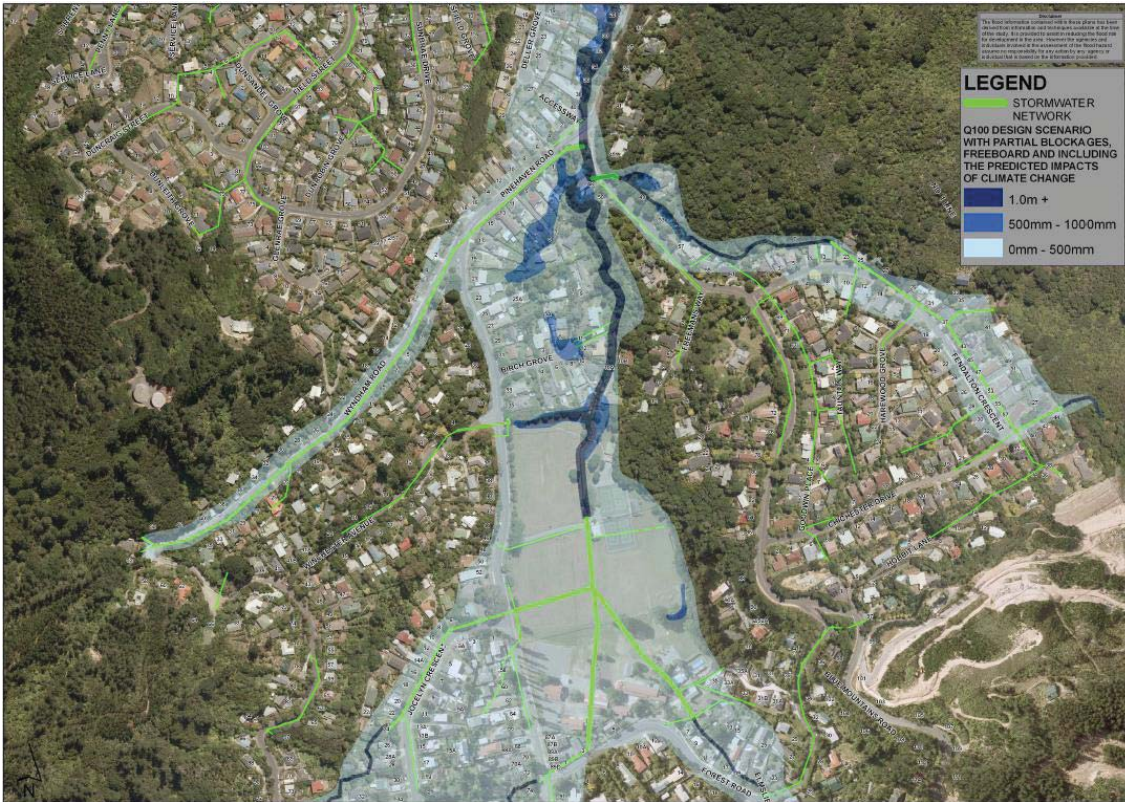
Figure 4.2 – Q100 design scenario including partial blockages, freeboard and predicted impacts of climate change
