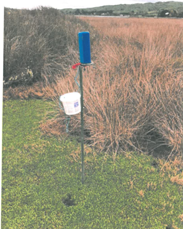
Photo B. "UE Boom 2" speaker on stand. Iphone in white container connected by blue speaker wire.
