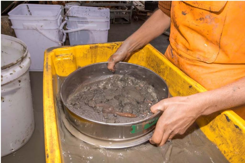
**Figure 5.4: NIWA laboratory technician sieving benthic sediment core samples to remove the bulk of fine sediment and mud for samples collected during the 2016 Wellington Harbour subtidal sediment survey**
