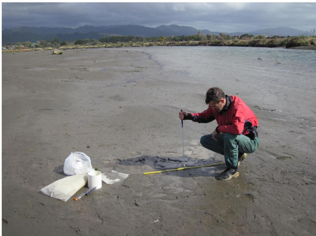
Figure 3.1: Sedimentation plate monitoring in the Waikanae Estuary, January 2017
