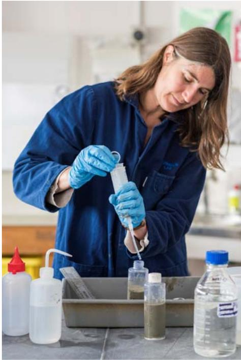
**Figure 5.3: NIWA laboratory technician siphoning off water from a sediment sample core bottle collected during the 2016 Wellington Harbour subtidal sediment survey**
