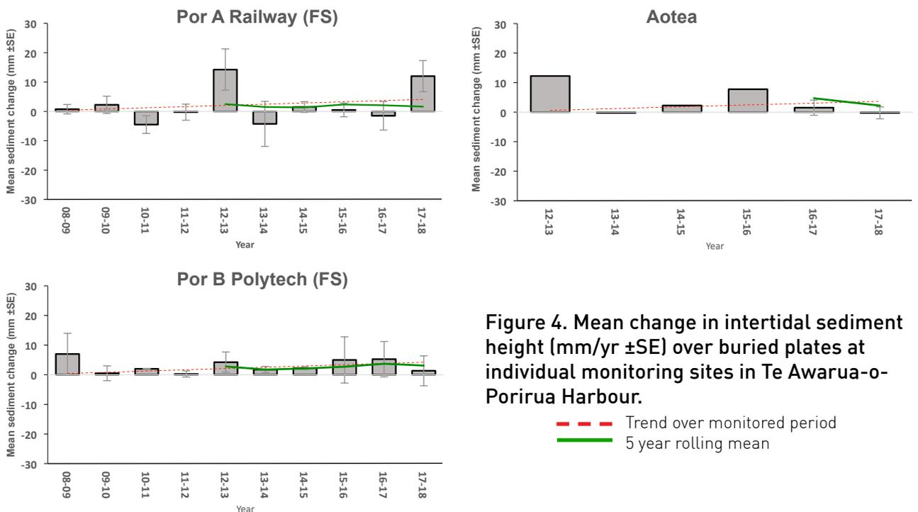
**Figure 4. Mean change in intertidal sediment height (mm/yr ±SE) over buried plates at individual monitoring sites in Te Awarua-o-Porirua Harbour.**
