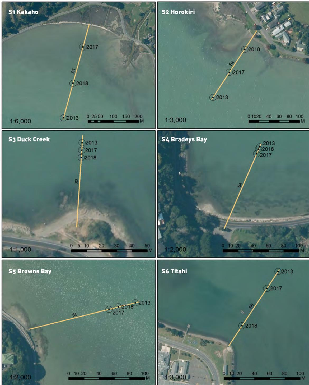
**Figure 2. Location of sediment transects used to measure the distance from subtidal plates to the soft mud boundary. The soft mud boundary in 2013, 2017, and 2018 is shown.**
