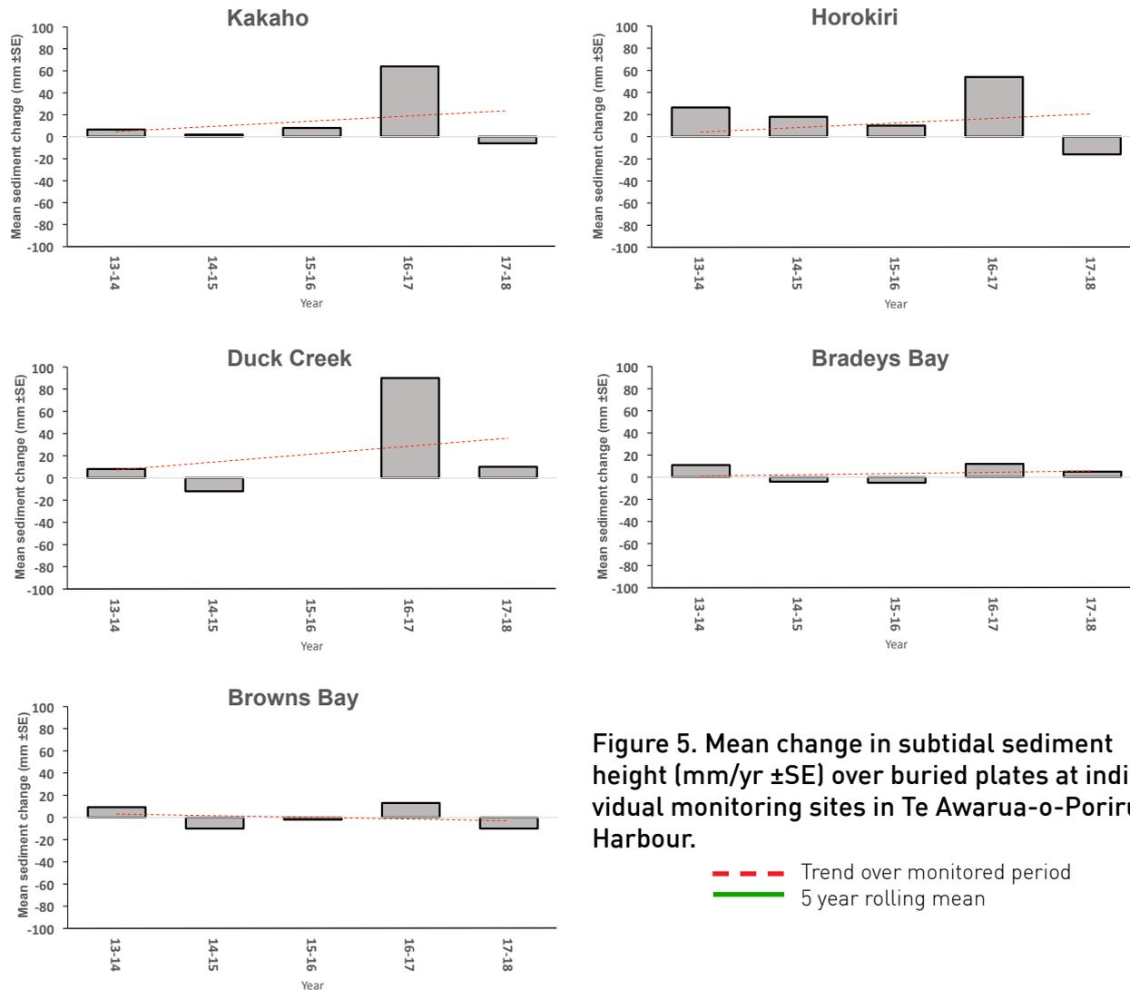
Figure 5. Mean change in subtidal sediment height (mm/yr ±SE) over buried plates at individual monitoring sites in Te Awarua-o-Porirua Harbour.
