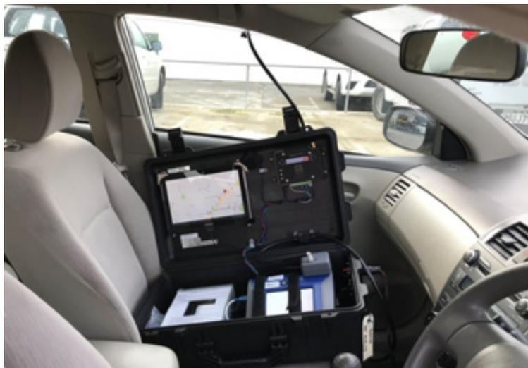
Figure 4.1: SmokeTrak measuring system set up in monitoring vehicle
