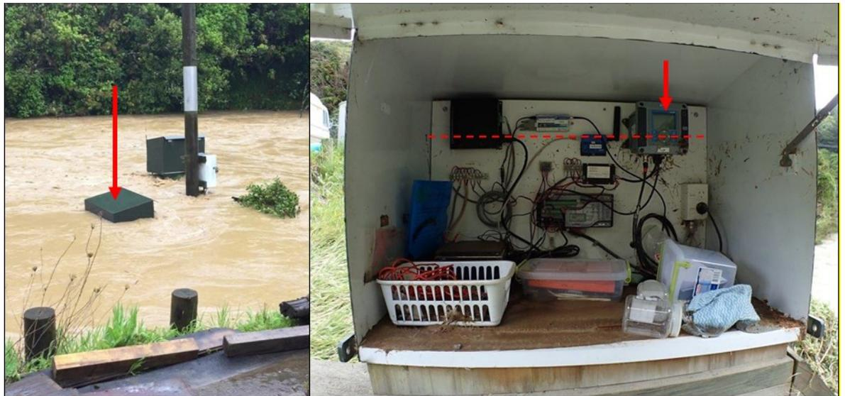
**Figure 3.10: Pauatahanui Stream at Gorge site during 14 November 2016 flood (left) showing station box with turbidity instrumentation (right) being flooded; dashed line is water level at peak of flood**
