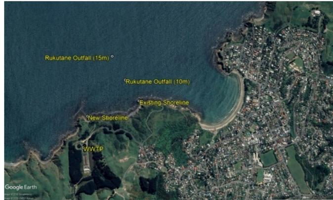
Figure 1. Location of existing WWTP shoreline discharge and alternative discharge options considered.
