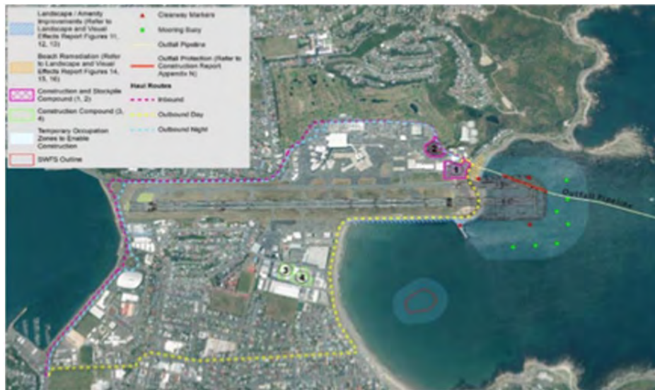
Figure 2: Reproduction of Figure 1.6 of the Resource Consents Application document showing what are referred to as Temporary Occupation Zones to Enable Construction (CMA areas appearing pale green/blue on aerial photo). These areas are referred to in paragraph 1.4.1 (p.10) as Temporary Exclusion Zones. The areas affected include both the areas of the proposed runway extension, and the location of the Submerged Wave Focussing Structure
