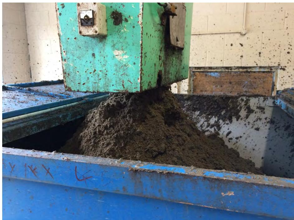
**Figure 9: Dewatered sludge awaiting covering and transport for landfill disposal**
