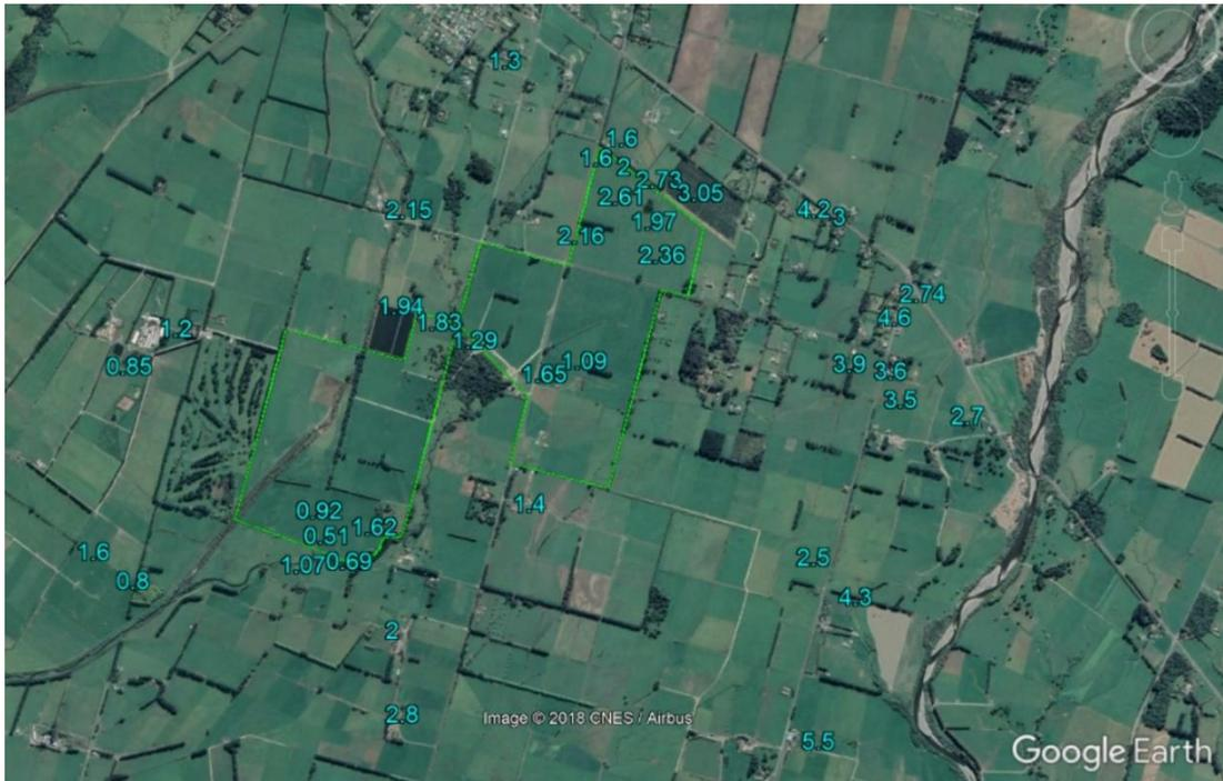
**Figure 6** Depth to Groundwater (m Below Ground Level)
