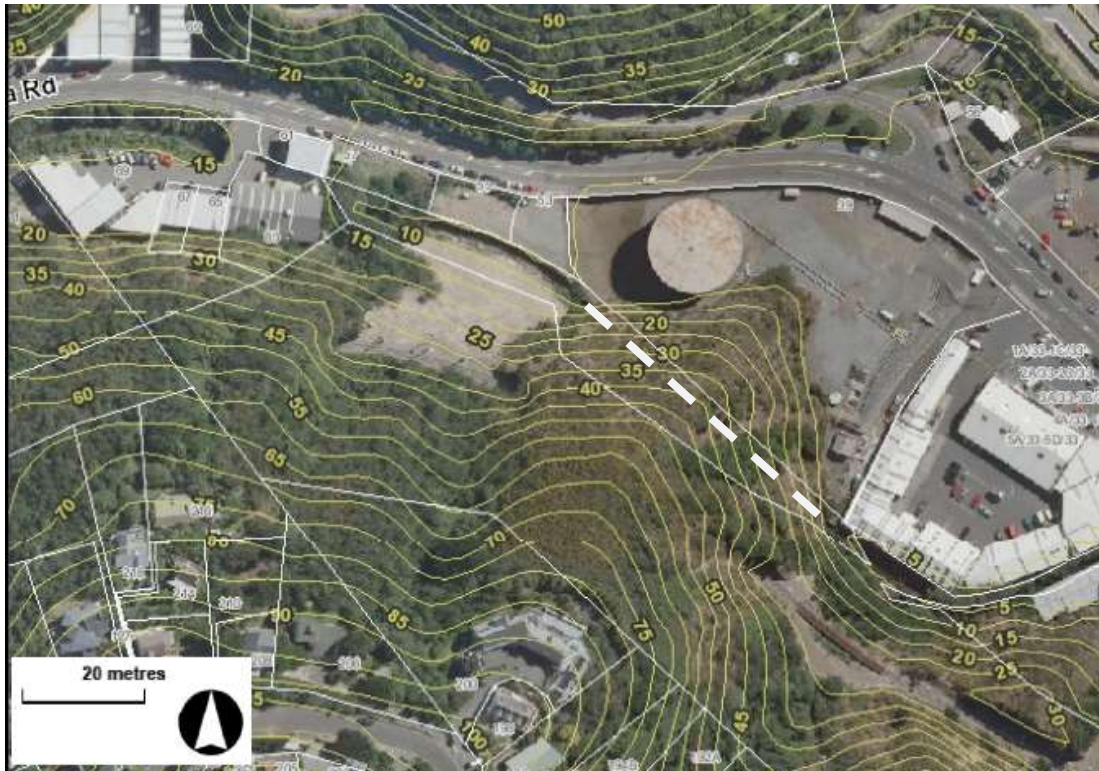
Aerial photography with 5-metre contours showing the location of the Kaiwharawhara stream diversion tunnel. (Source Wellington City Council on-line GIS, 2015)
