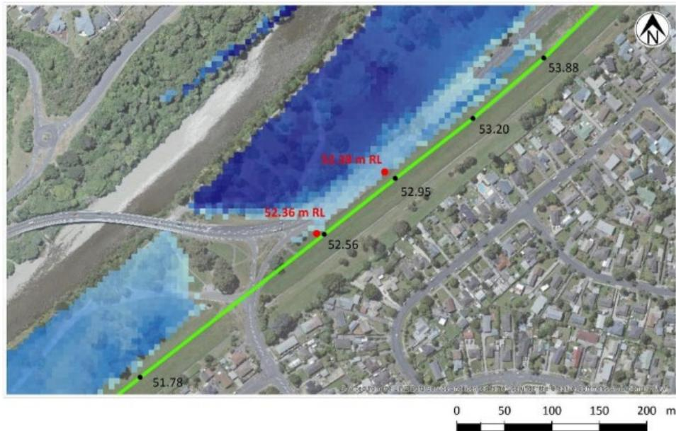
Figure 2 – Peak water levels in the 1 in 440 or the 2,300 cumec event
