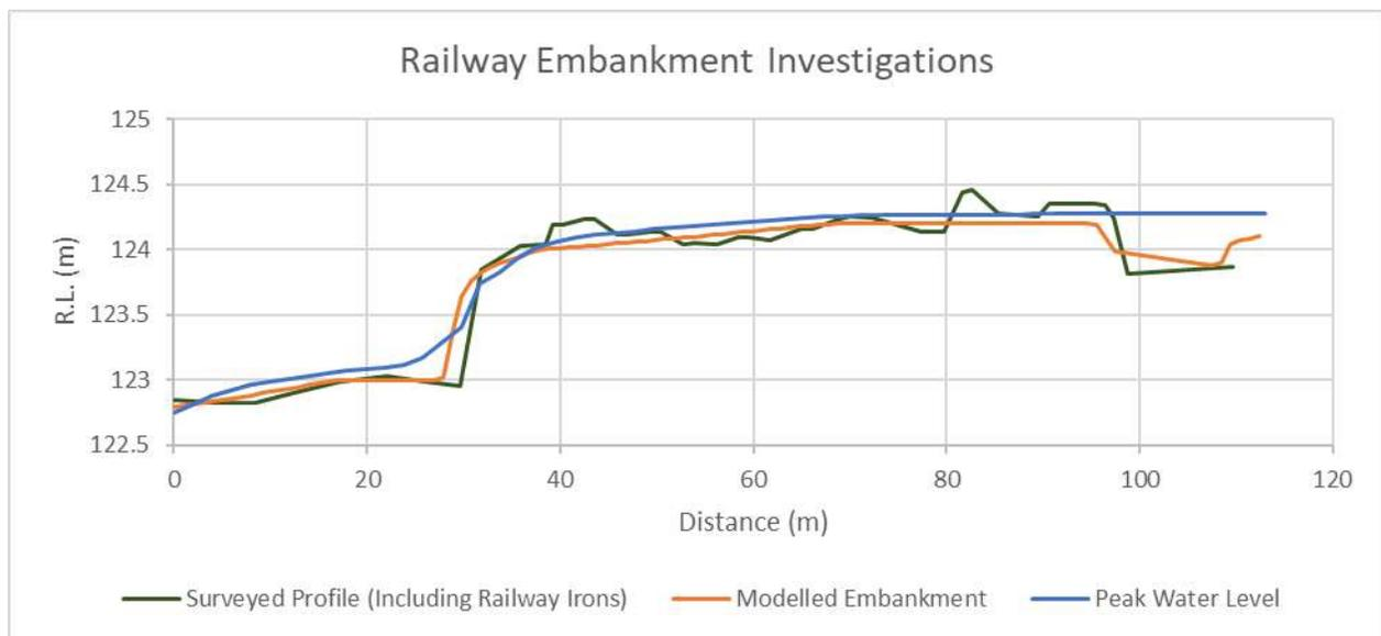
**Figure 7-25 – Comparison of modelled embankment levels with survey**
