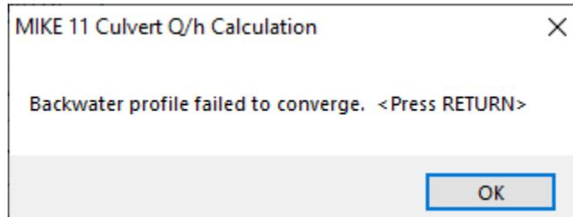
This indicates that the bridge setup in this location needs to be refined in order to function correctly. (Discussions with Susan Borrer have indicated that this cannot be replicated in house and maybe due to a version issue with the software. My checks have been carried out using the 2017 SP2 version of the software – the results still show a minor instability however).
