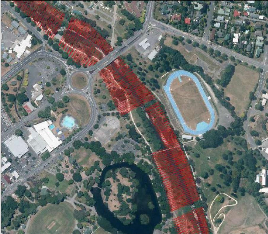
Figure 7-18 – Visualisation of lateral link connections showing gap in right bank lateral link (red lines showing link connections to centre of river)
