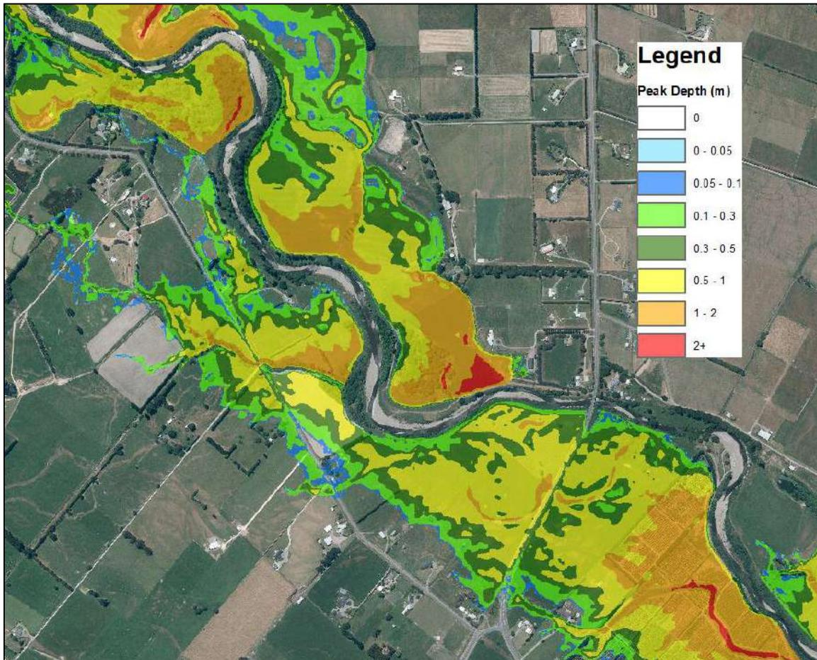
Figure 4-1 - Example of colour scheme used in recent Waiohine River modelling
