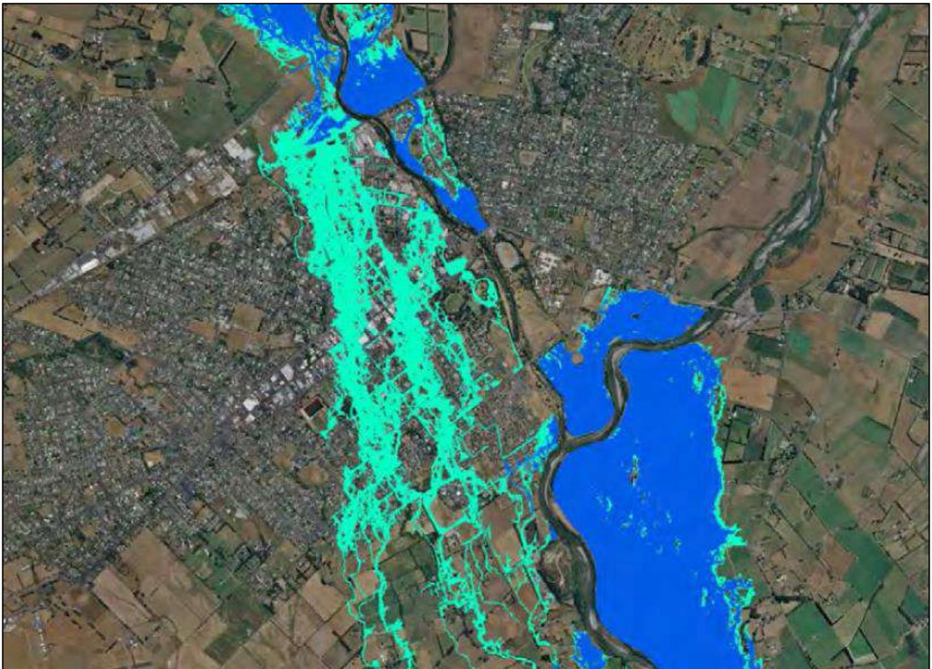
**Figure 7-2 – Modelled flood extent showing flood waters overtopping the railway embankment**
