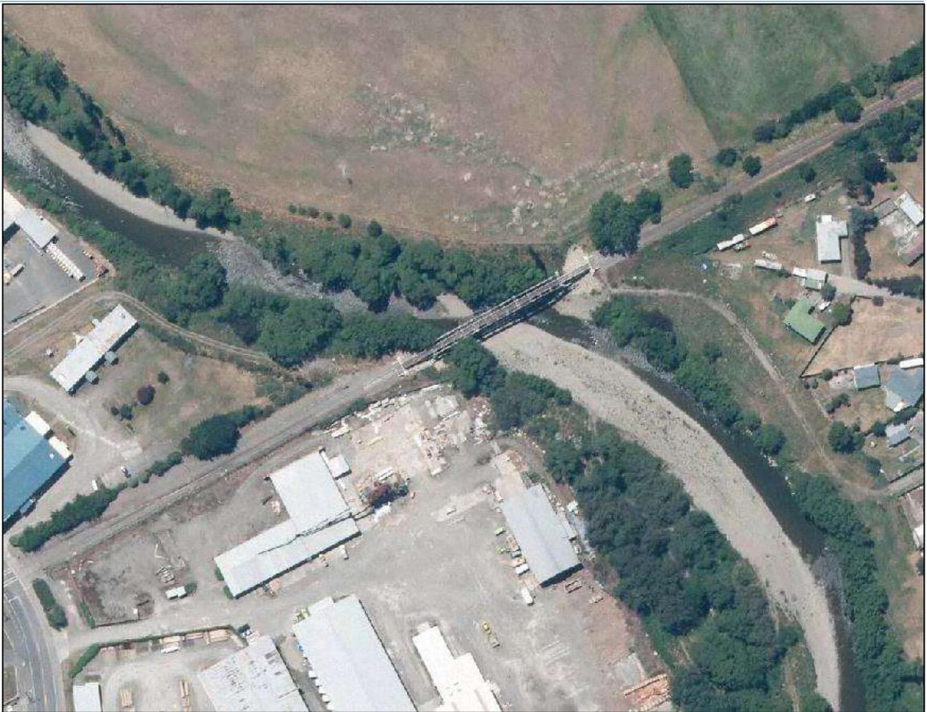
Figure 7-4 – Aerial Image of railway bridge showing skewed alignment
