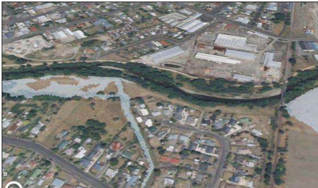
Figure 7-8 – 1998 calibration model results showing ponding on left bank upstream of railway bridge
