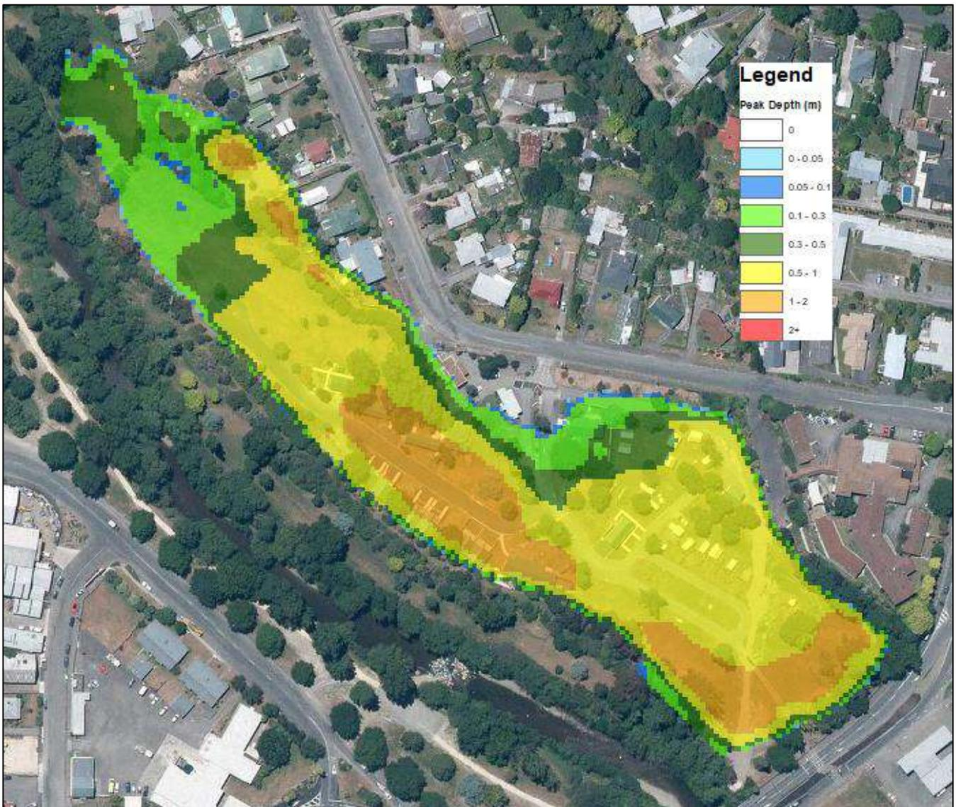
Figure 7-20 - 1998 Calibration results showing water depths
