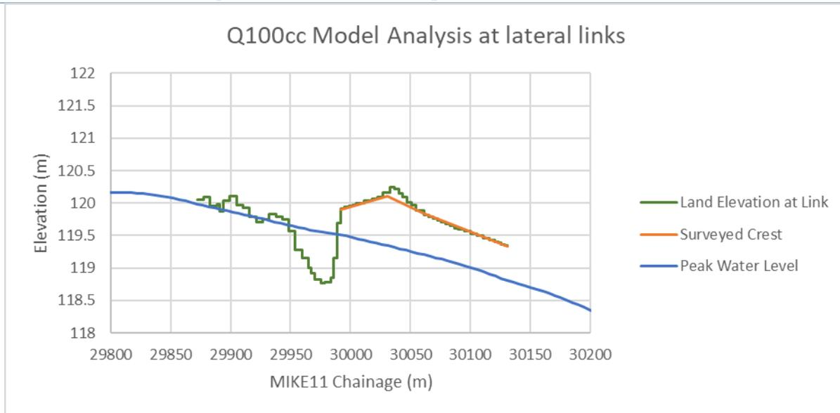
**Figure 7-21 – Inspection of modelled links at left bank spill location**
