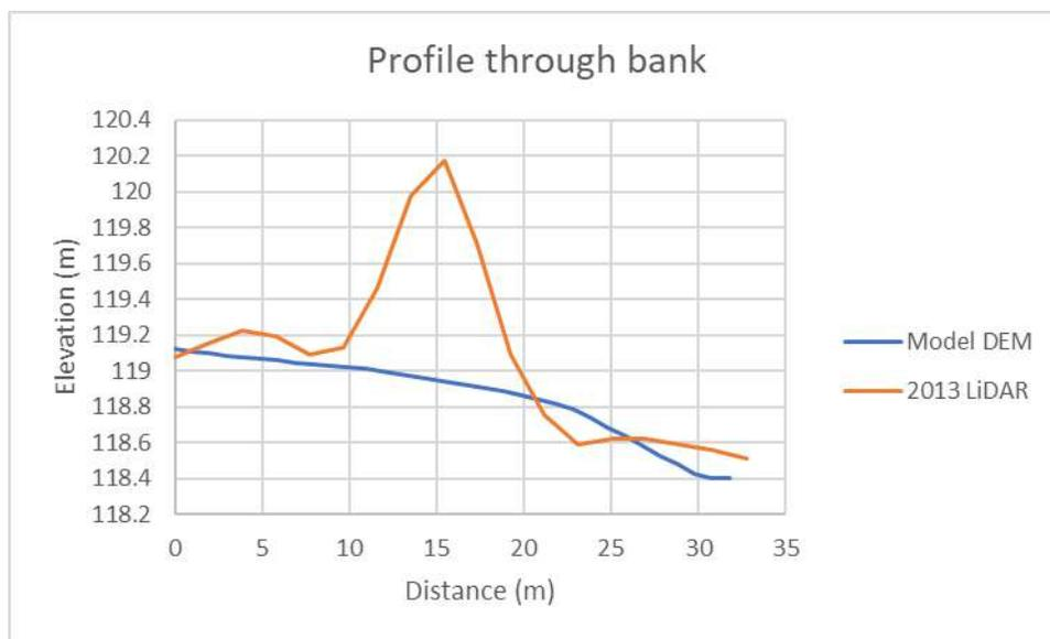
**Figure 7-22 – Comparison of modelled terrain levels (2008 LiDAR) with 2013 LiDAR**
