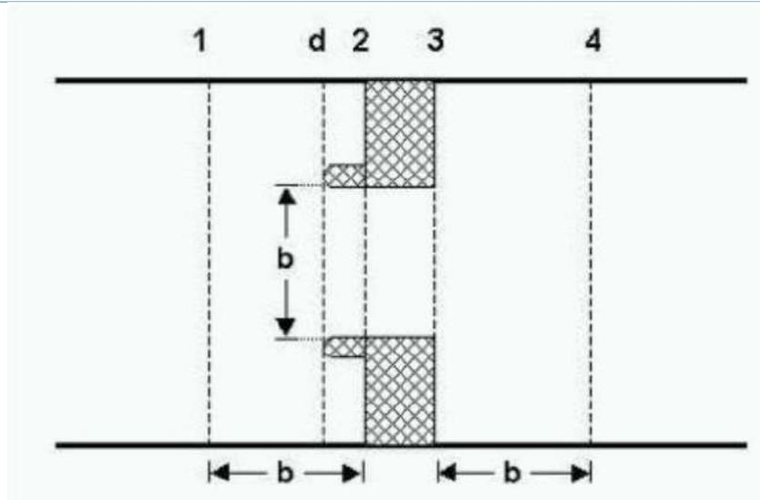
Figure 5-4 - Location of cross sections for FHWA WSPRO bridge method (M11 reference manual)
