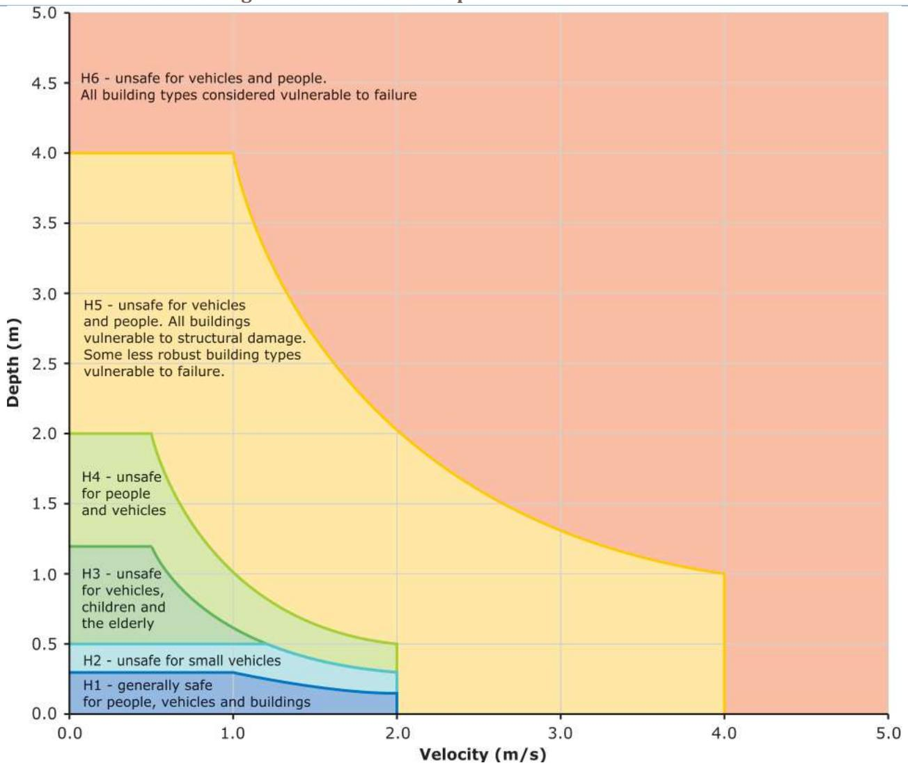
Figure 4-2 - Graphical representation of the Hazard Categories
