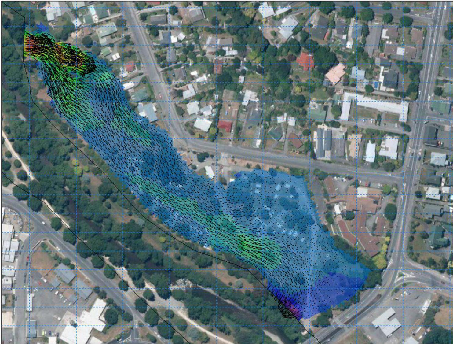
Figure 7-19 - 1998 Calibration results overlaid with vectors showing the direction of flow
