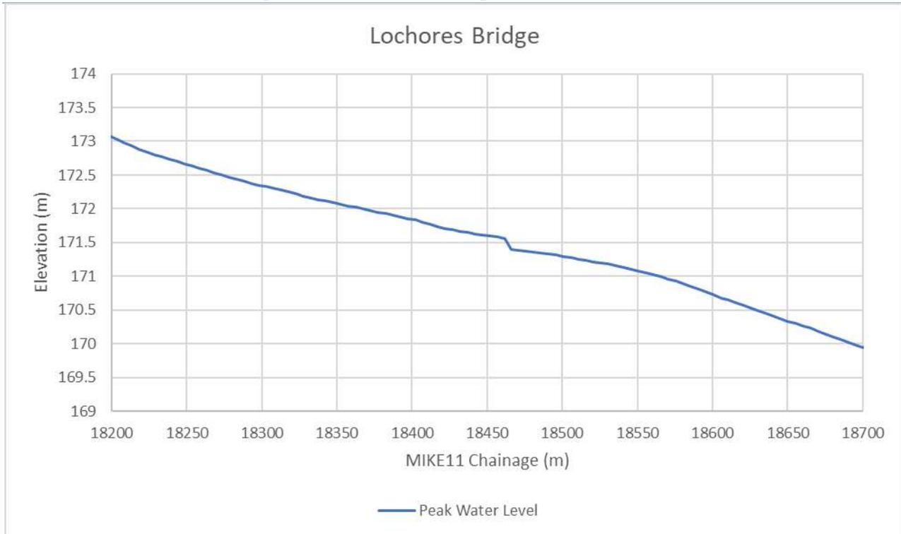
**Figure 7-17 - Observed headloss through Lochores Rd Bridge (50 year CC)**
