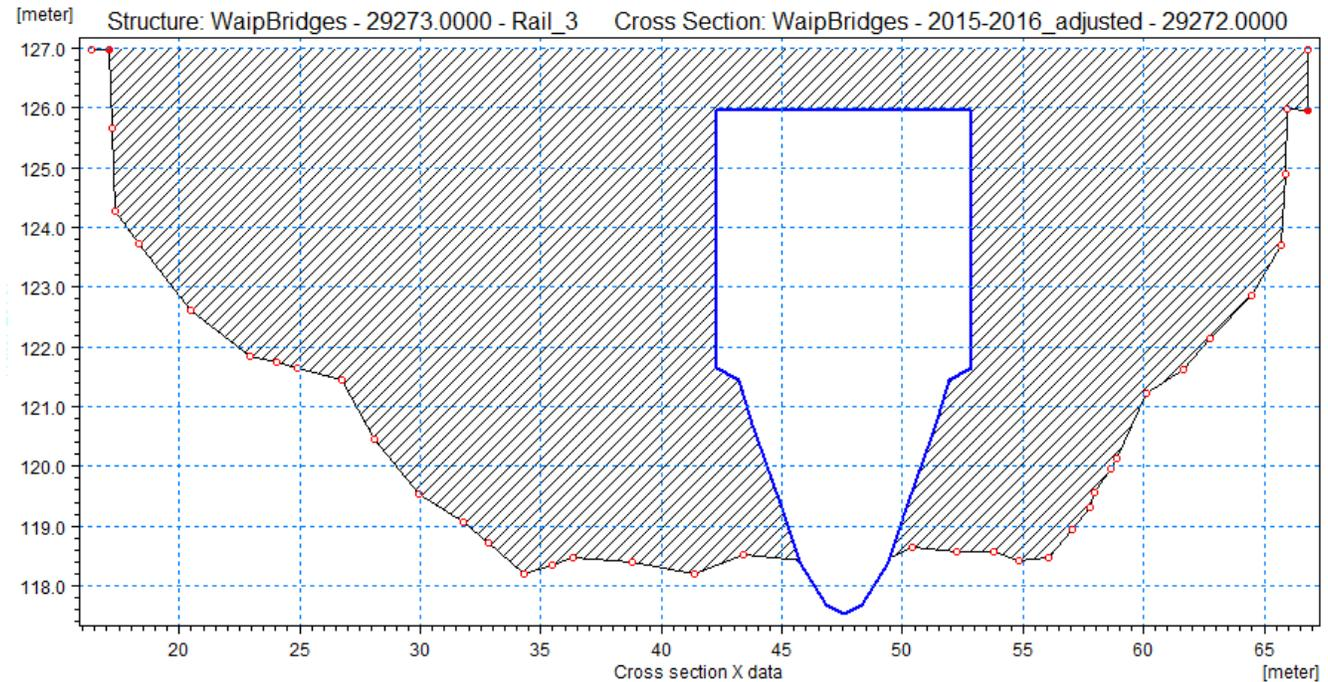
**Figure 7-5 – Visualisation of modelled representation of individual rail bridge span.**
