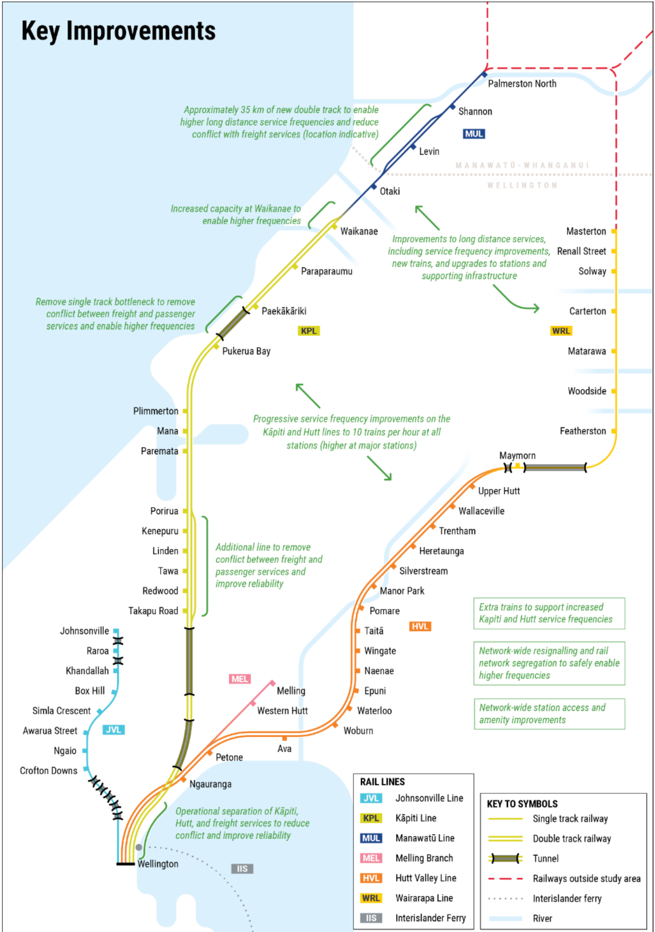
Figure 17: Planned improvements to rail infrastructure
