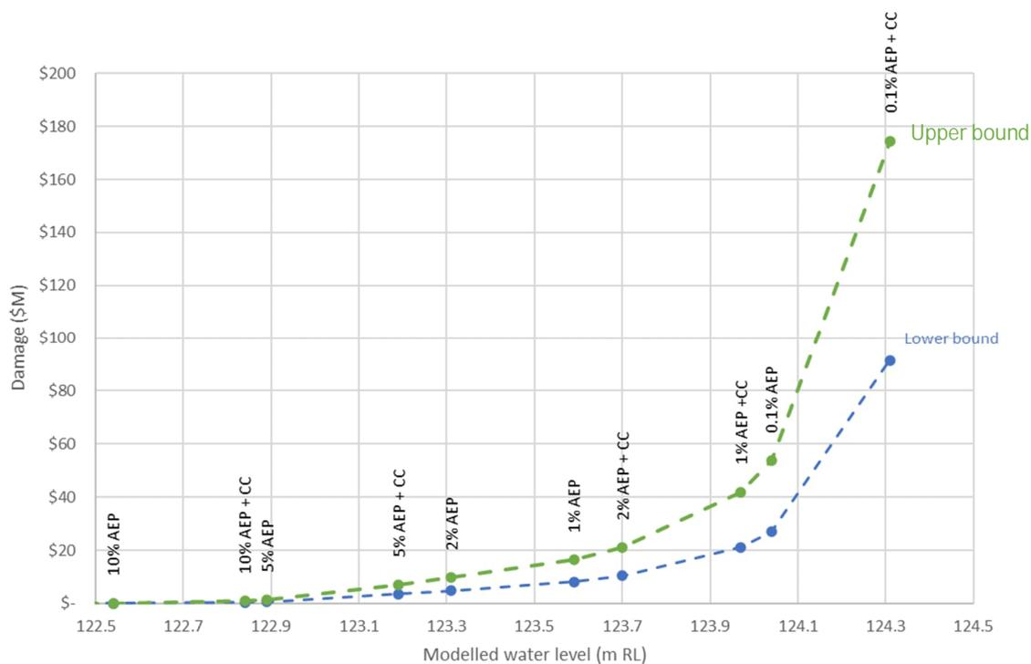
Figure 5.1 Stage-damage curves at the railway bridge
