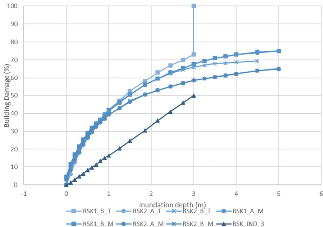
Figure 4.1: Fragility functions used in this assessment for buildings (residential, commercial and industrial) (NIWA, 2010).
