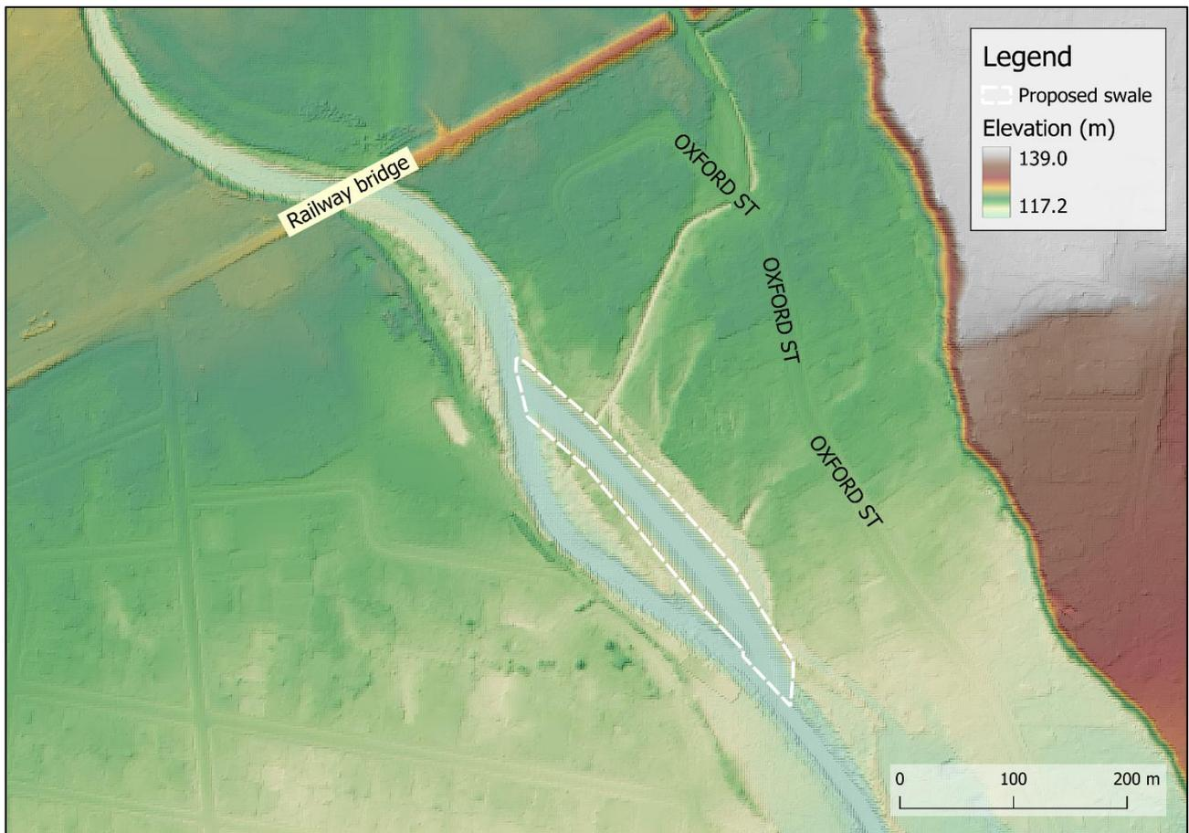
**Figure 3-28: Option 21 swale location near Oxford St**
