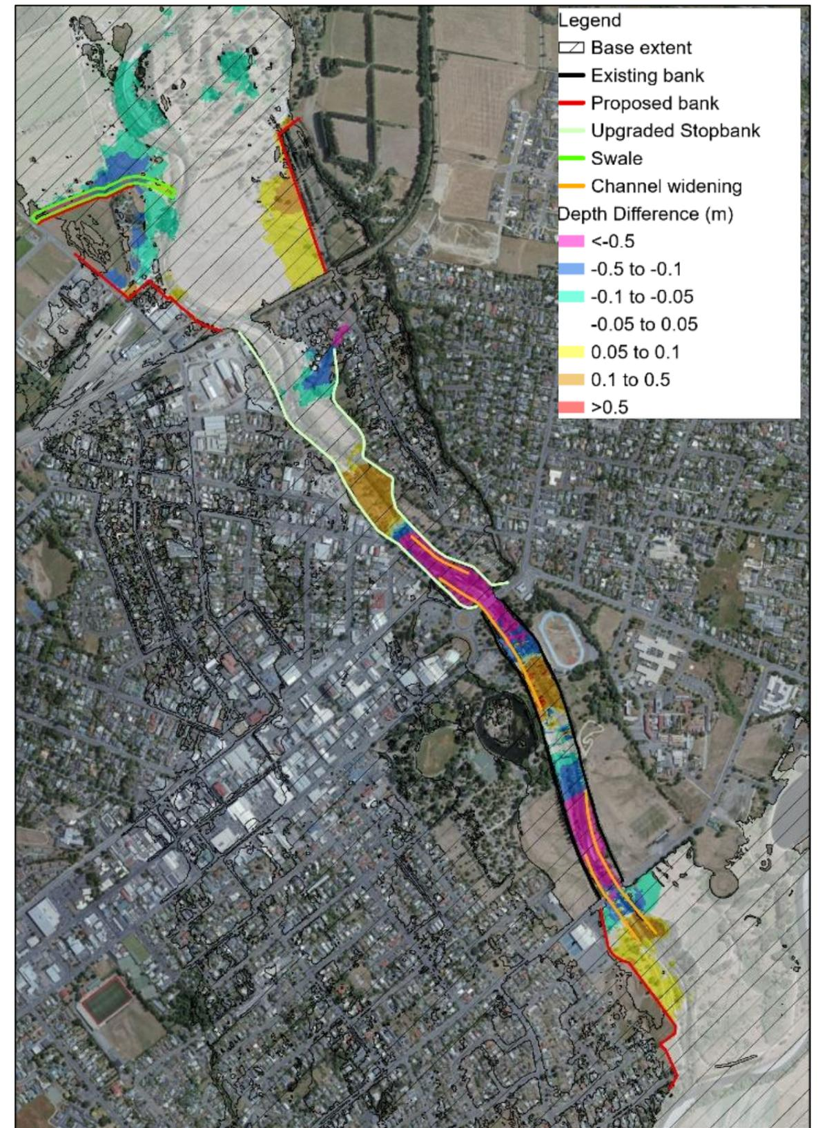
Figure 3-80: Final Iteration Option 4 depth difference map
