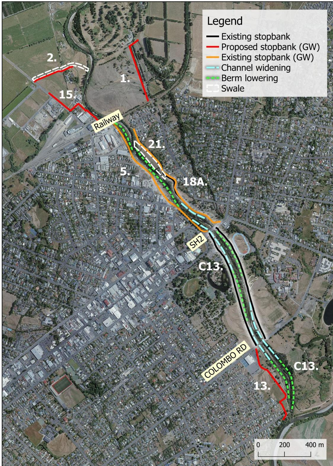
Figure 3-83: Final Iteration Option 2
