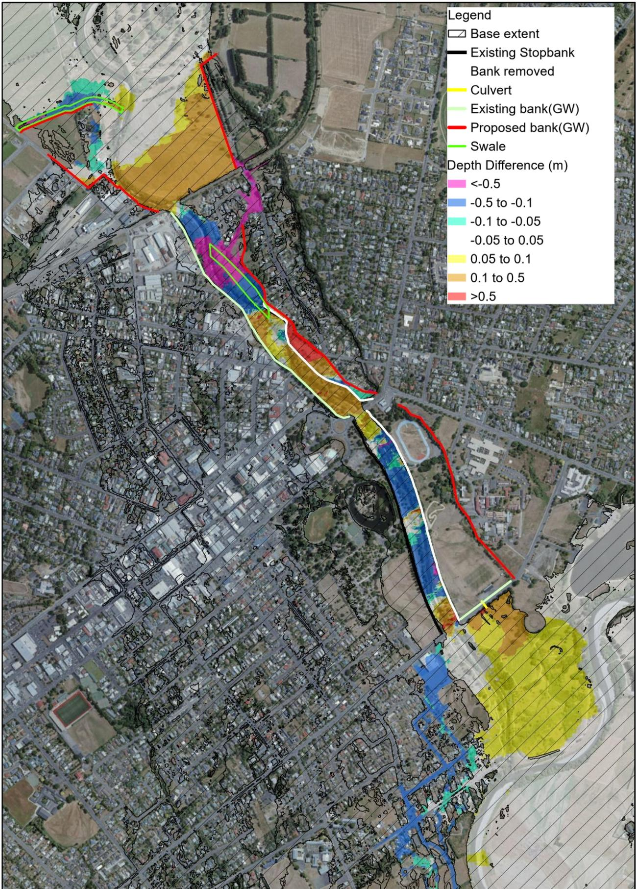
Figure 3-59: Combined Option 9 depth difference map (with bund at Akura).
