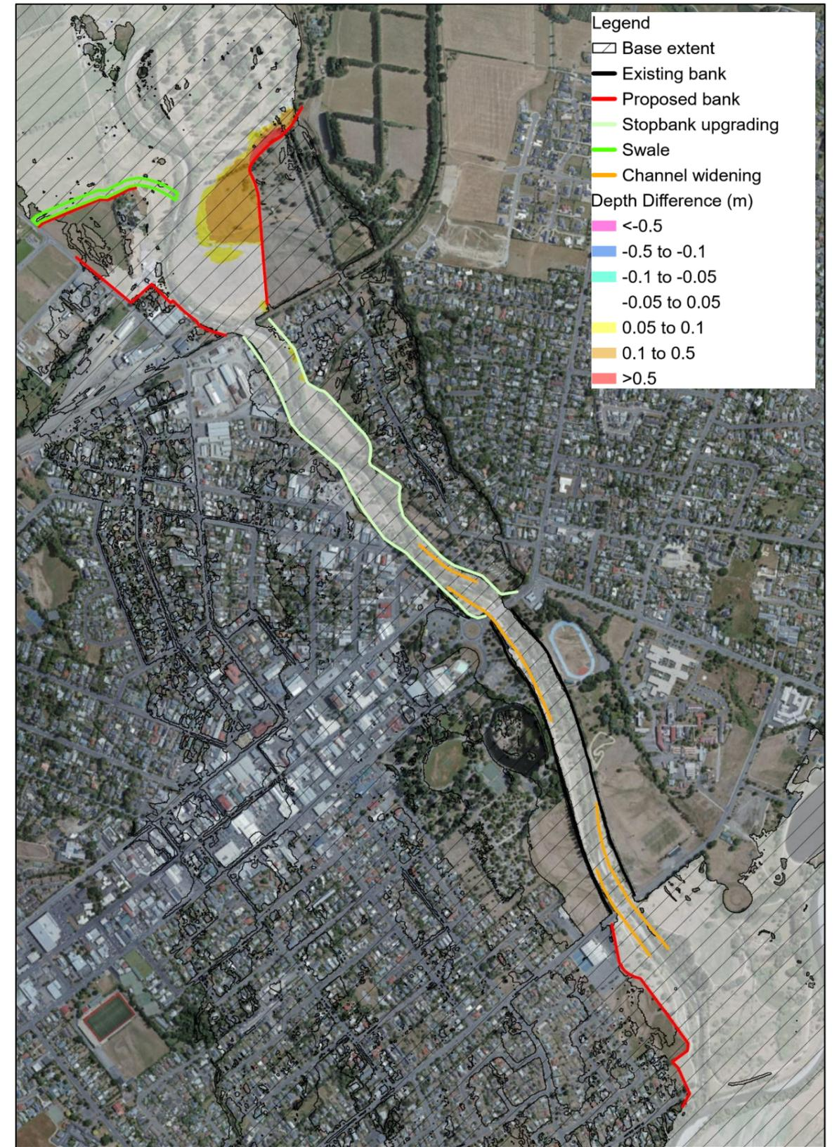
Figure 3-82: Final Iteration Option 6 depth difference map with Final Iteration Option 1B
