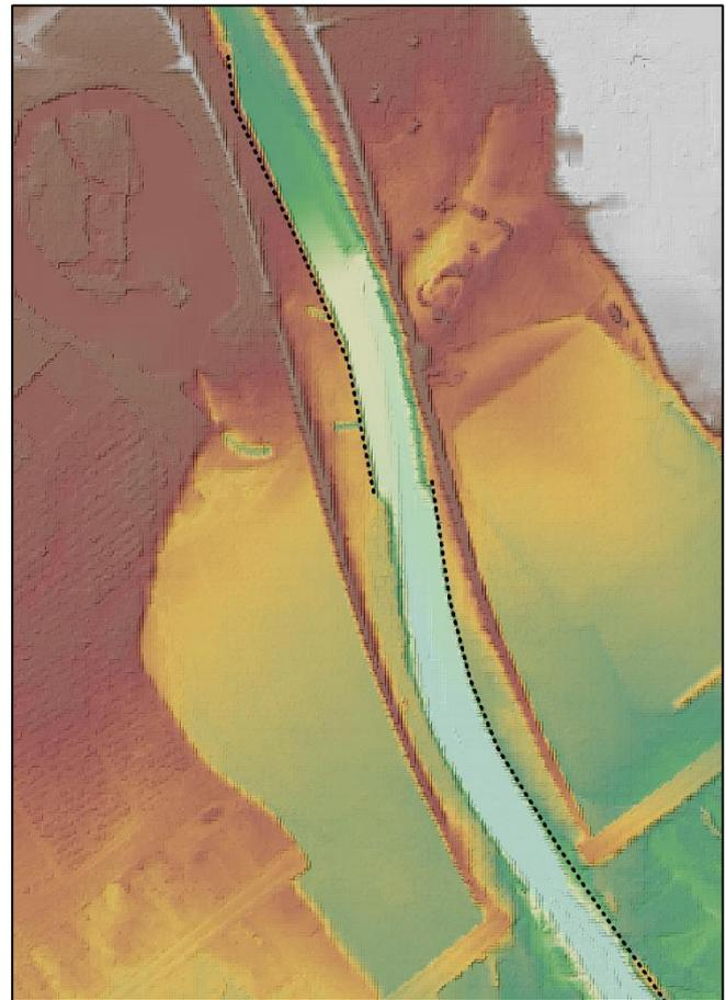
**Figure 3-42: Option 22 DEM with widened channel burnt in**
