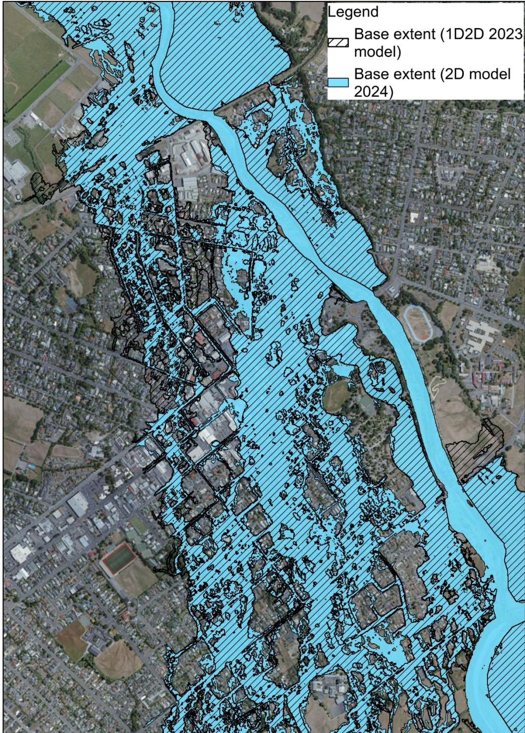
**Figure 2-3: The 2D Waipoua Model flood extent for the base scenario (status quo) and a 1% RCP6.0 flow event, compared to the 2023 Waipoua Hydraulic Model**
