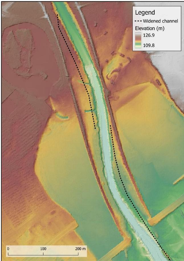
**Figure 3-41: Base scenario DEM with Option 22 widened channel indicated (dashed line)**
