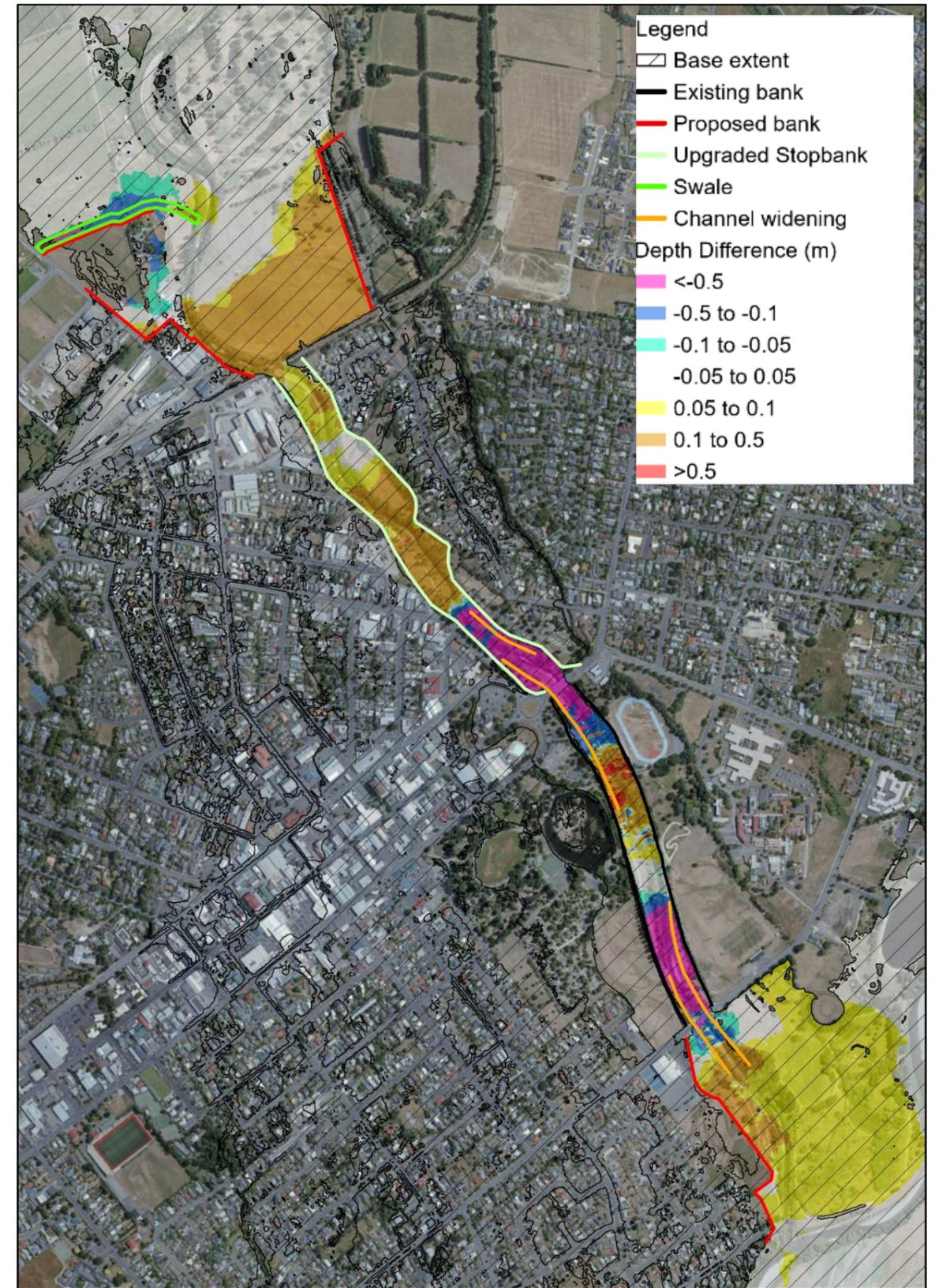
Figure 3-78: Final Iteration Option 1B depth difference map (Mawley Park stopbank extension).
