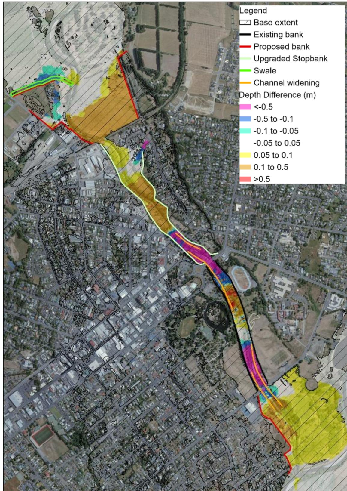
Figure 3-91: Final Iteration 1 depth difference map.
