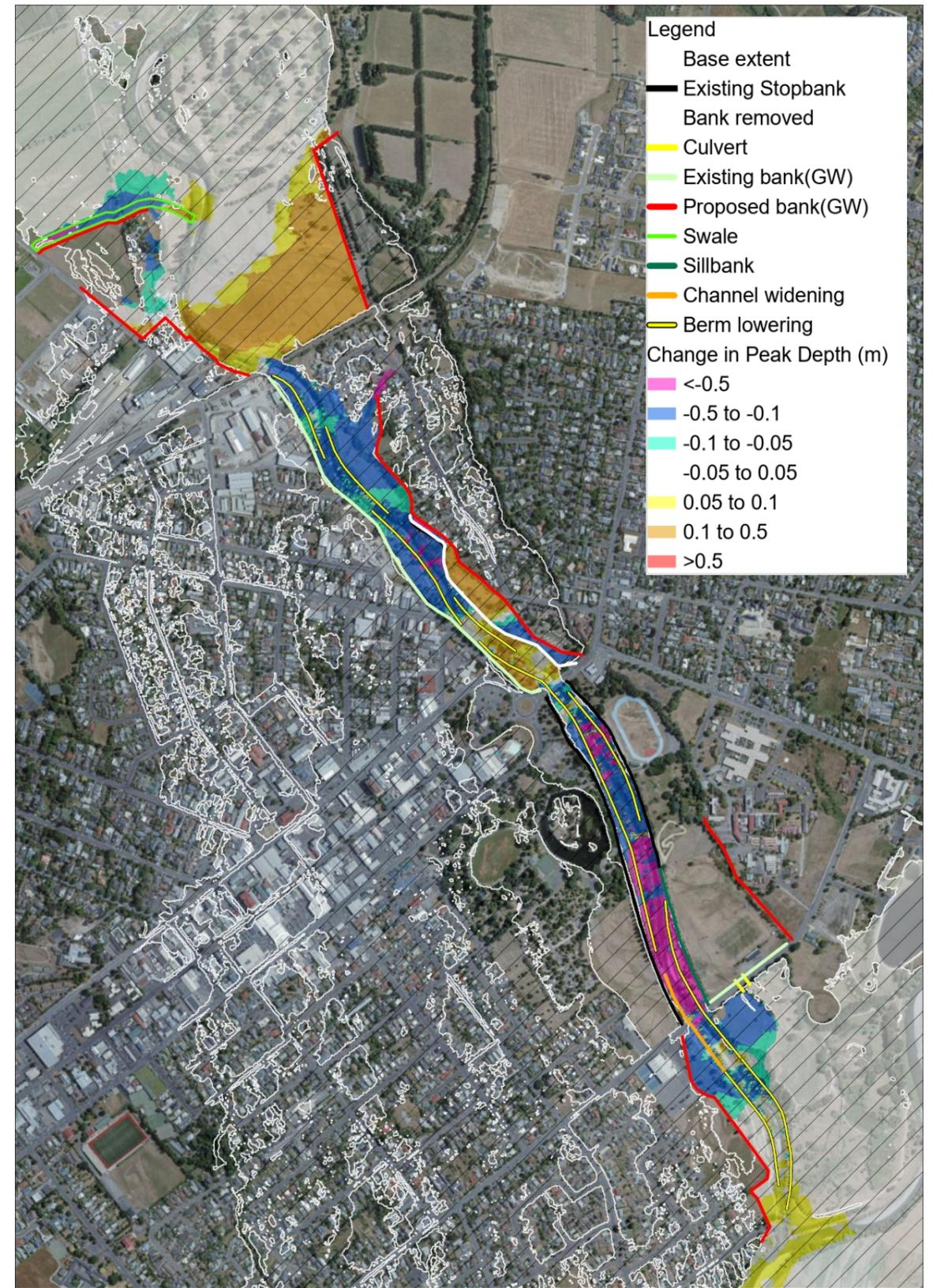
Figure 3-72: Combined Option 14B depth difference map (with bund at Railway bridge).
