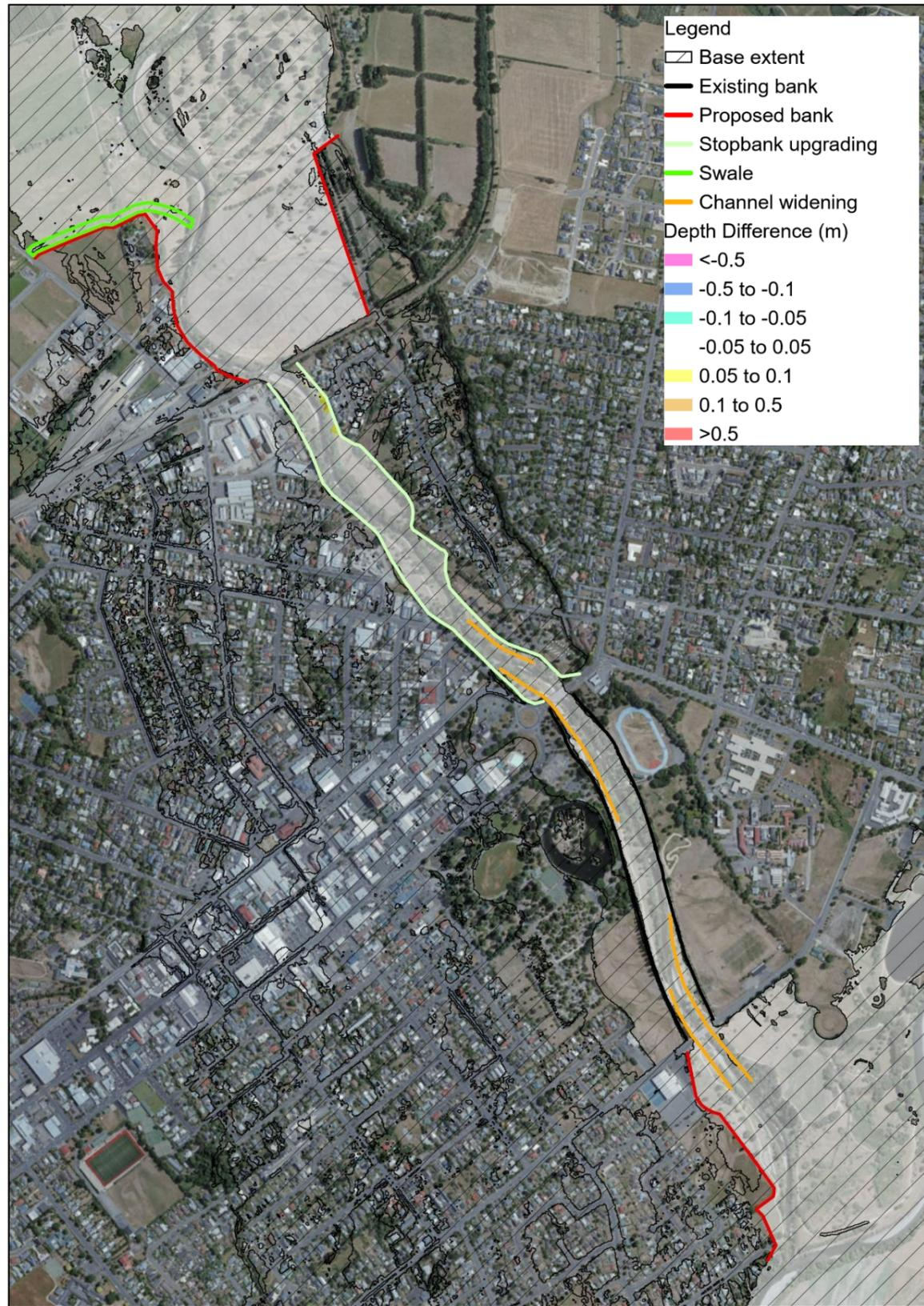
Figure 3-81: Final Iteration Option 5 depth difference with Final Iteration Option 1B
