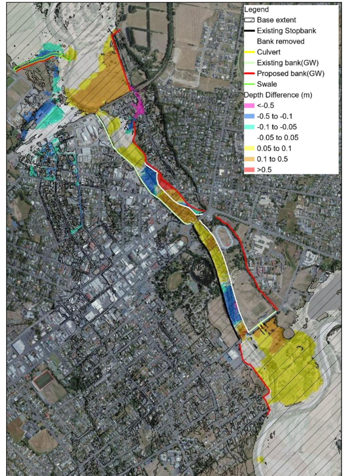
Figure 3-65: Combined Option 11B depth difference map (without swale at Oxford St).
