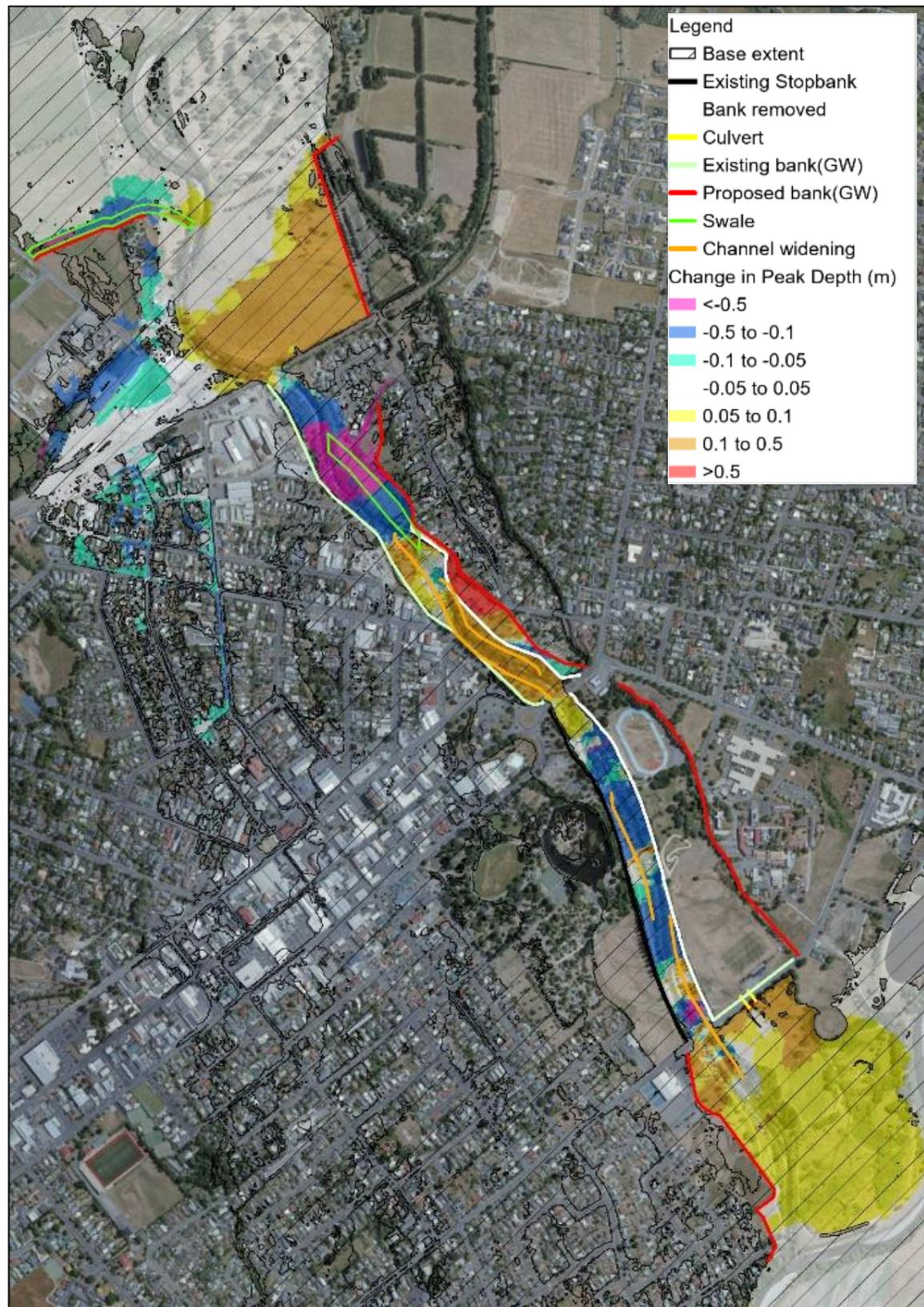
Figure 3-66: Combined Option 12 depth difference map (with swale at Oxford St).
