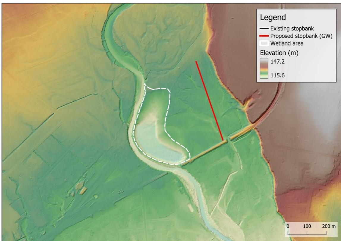
Figure 3-2: Option 1A (without an inlet to Mahunga wetland)
