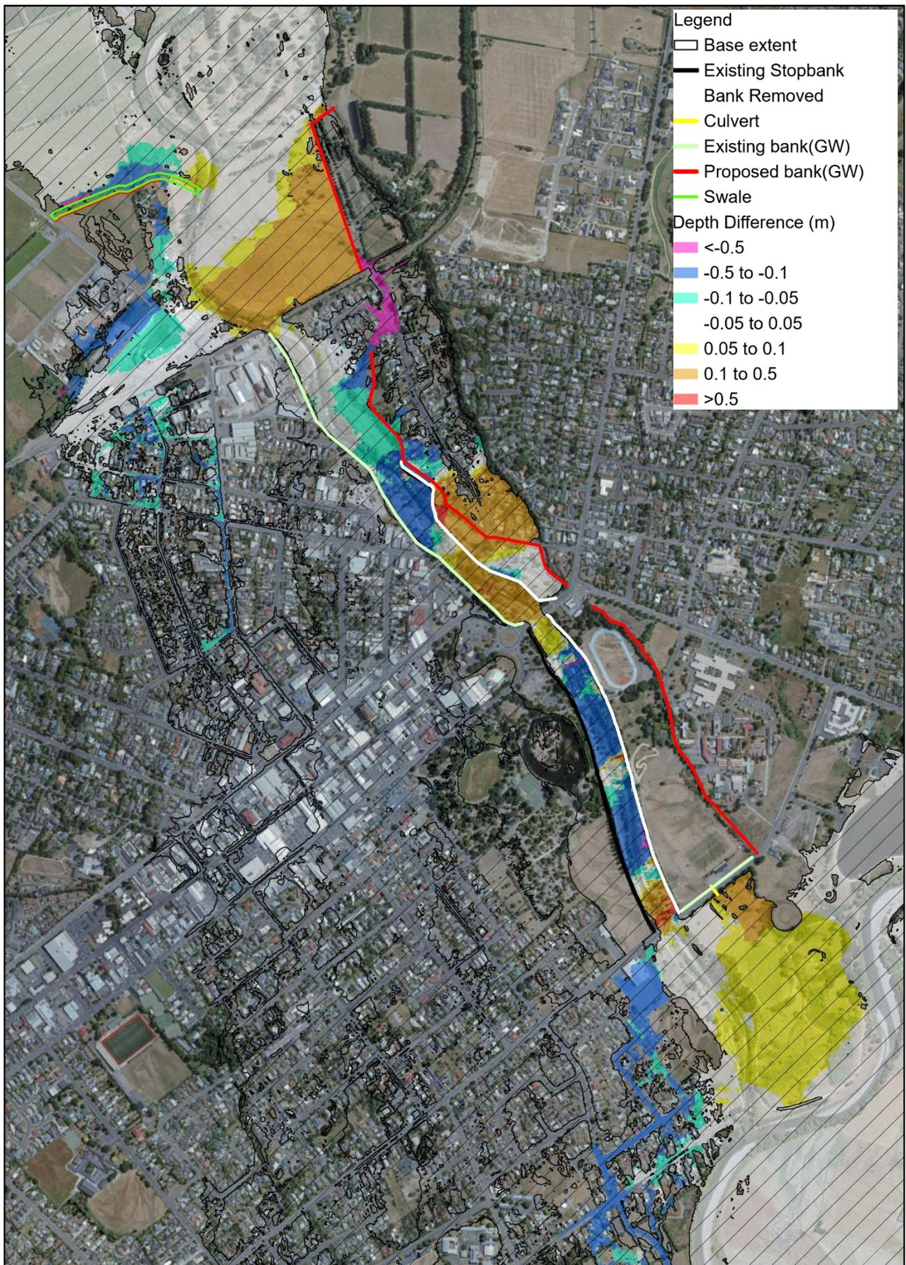
Figure 3-50: Combined Option 3 depth difference map (with bund at Akura).
