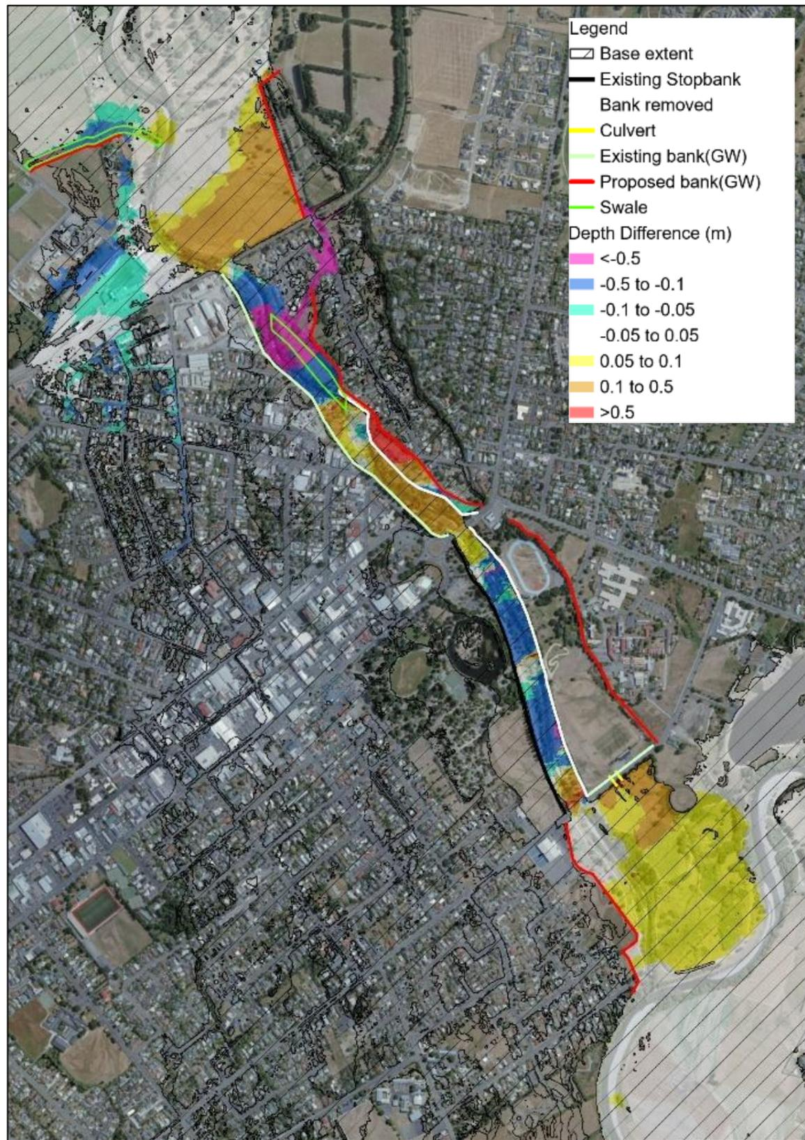
Figure 3-64: Combined Option 11A depth difference map (with swale at Oxford St).
