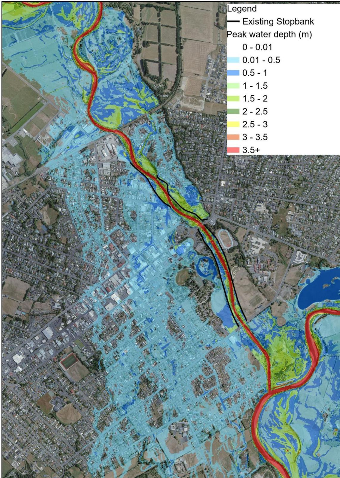
Figure 3-1: Base scenario (existing scheme) 1% AEP RCP6.0 depth map
