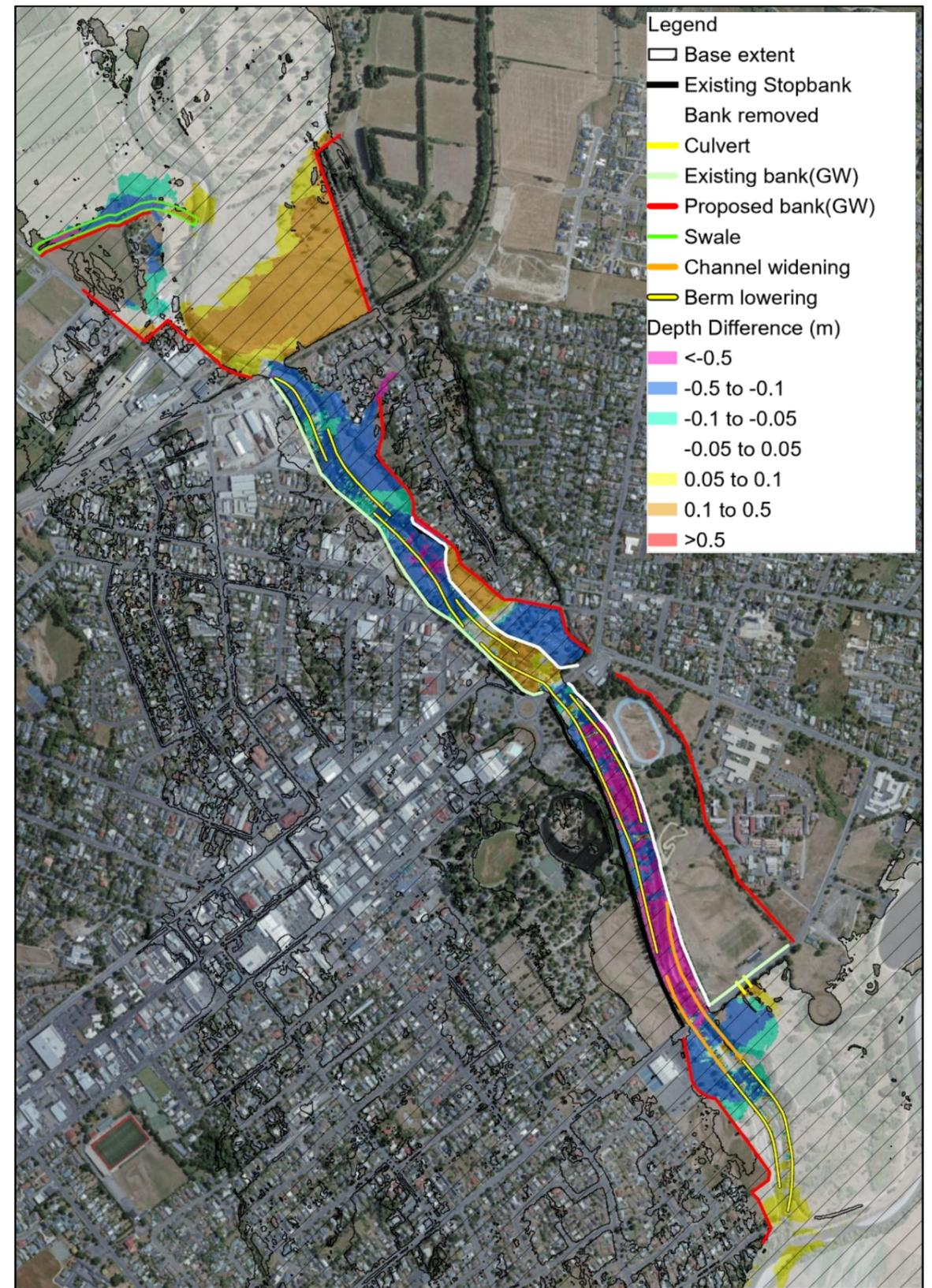
Figure 3-74: Combined Option 15 depth difference map (with bund at Railway bridge).
