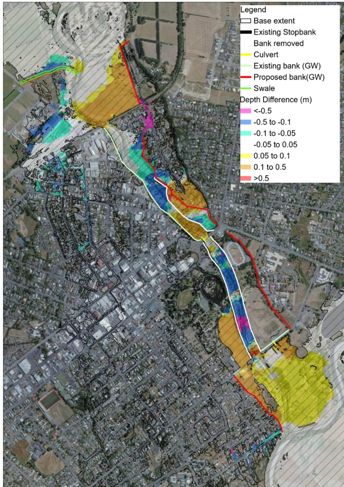
Figure 3-52: Combined Option 4 depth difference map (with bund at Akura).
