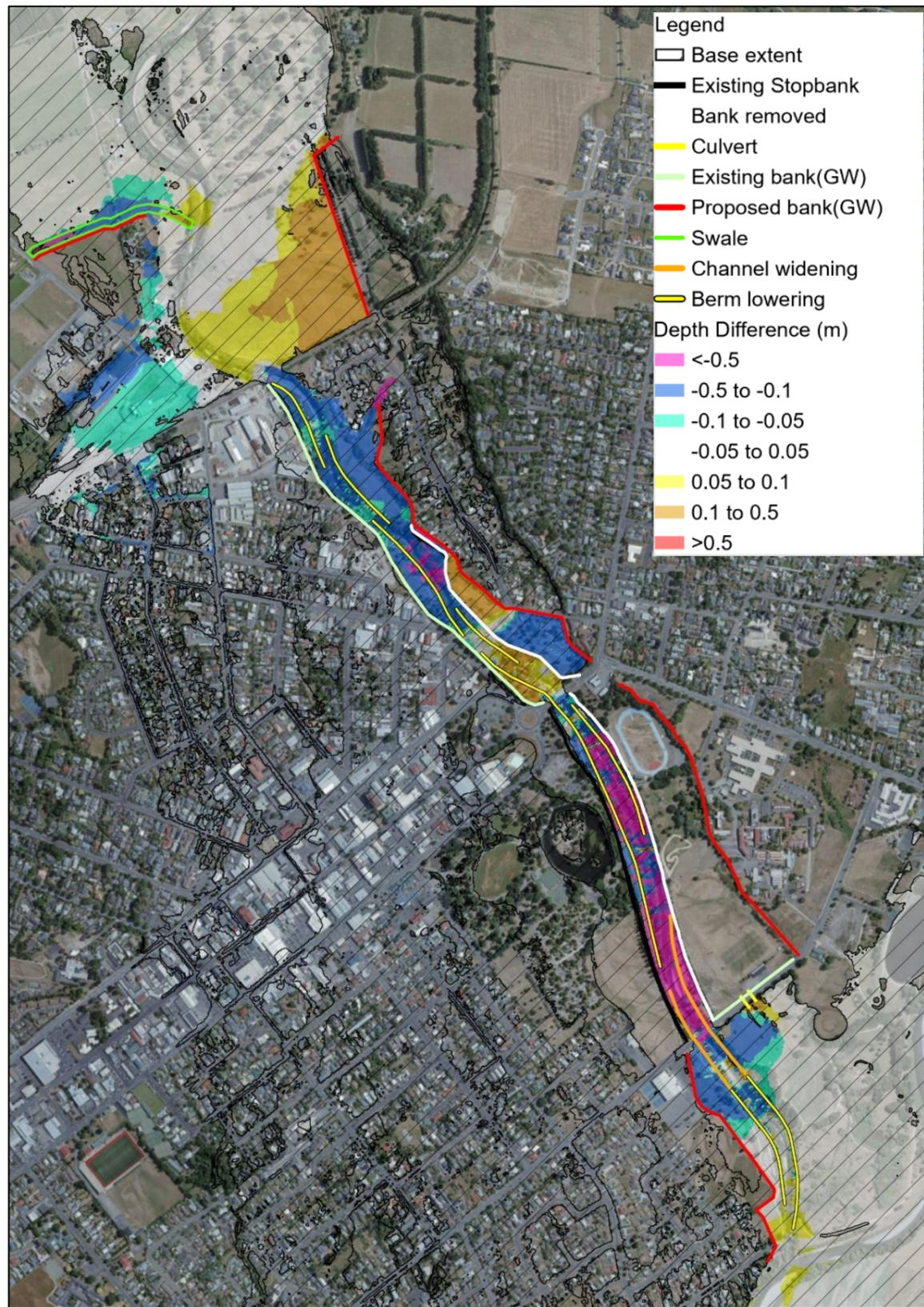
Figure 3-73: Combined Option 15 depth difference map (without bund at Railway bridge).
