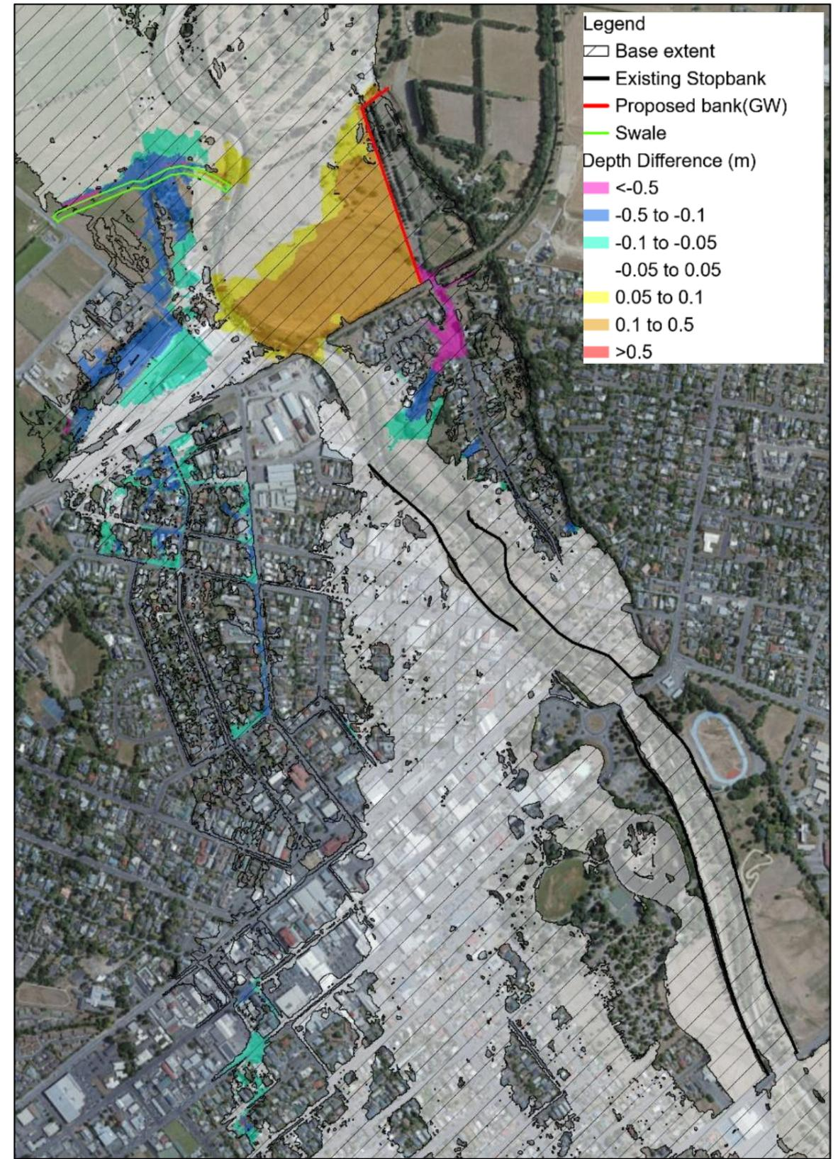
Figure 3-46: Combined Option 1B depth difference map (without bund at Akura Rd swale).
