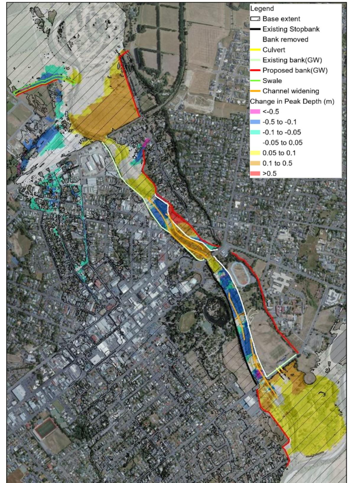
Figure 3-67: Combined Option 12 depth difference map (without swale at Oxford St).
