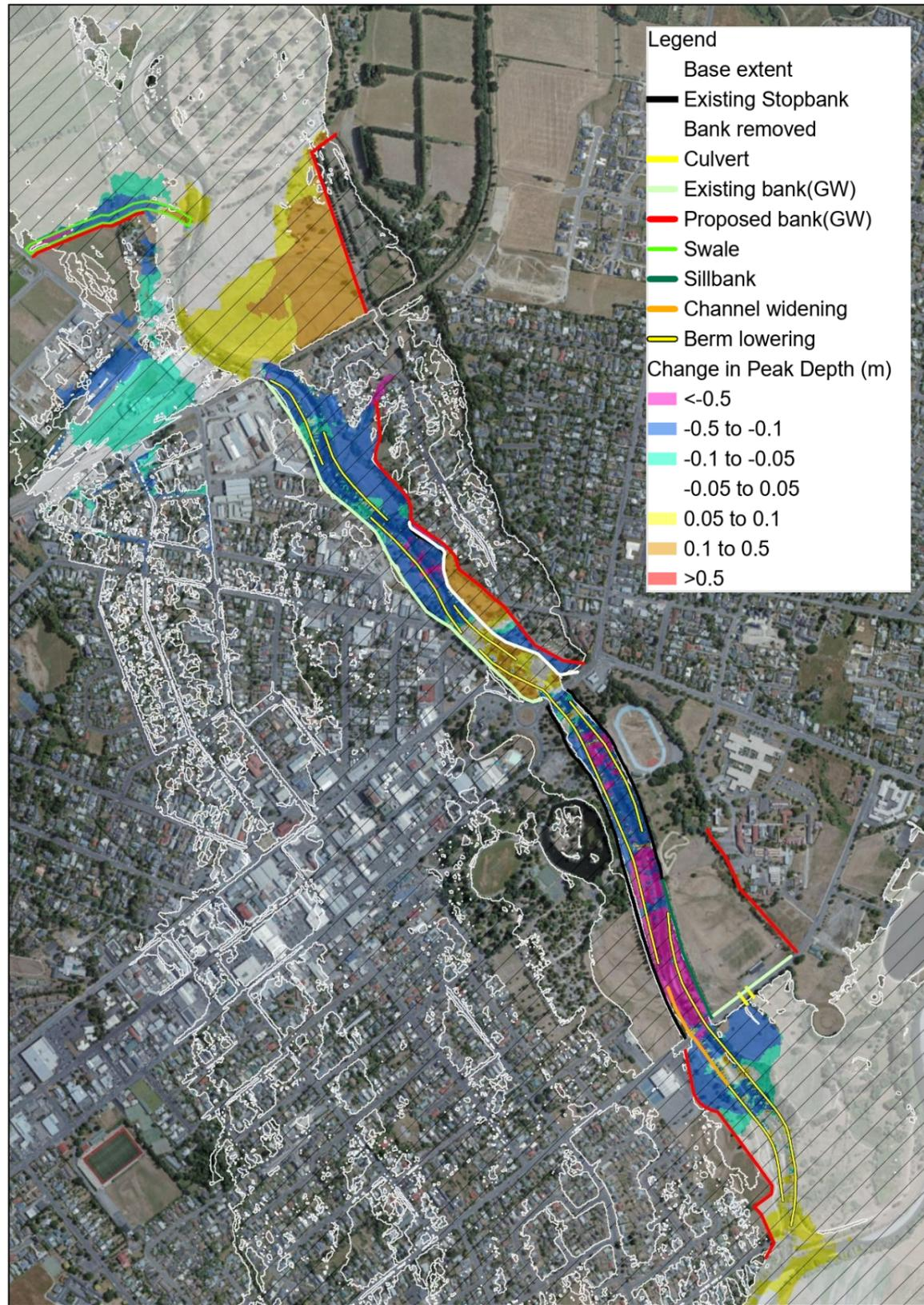
Figure 3-71: Combined Option 14A depth difference map (without bund at Railway bridge).
