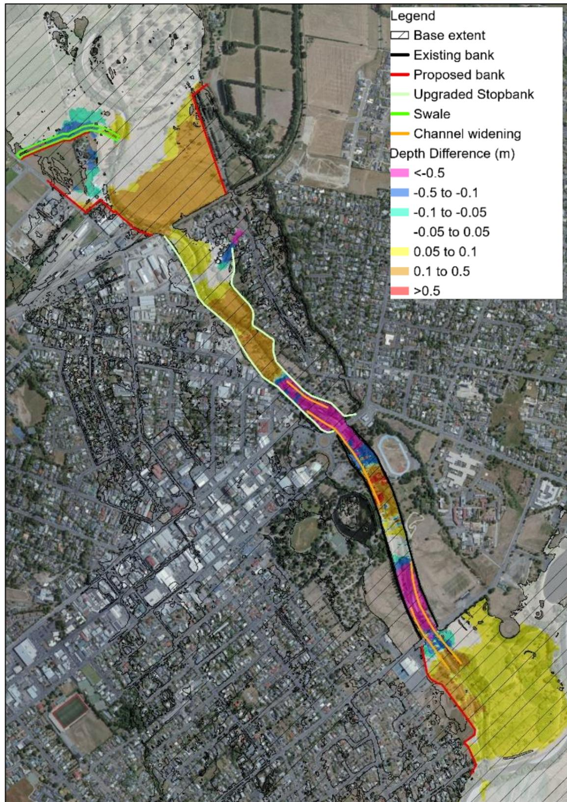
Figure 3-79: Final Iteration Option 1 depth difference map.
