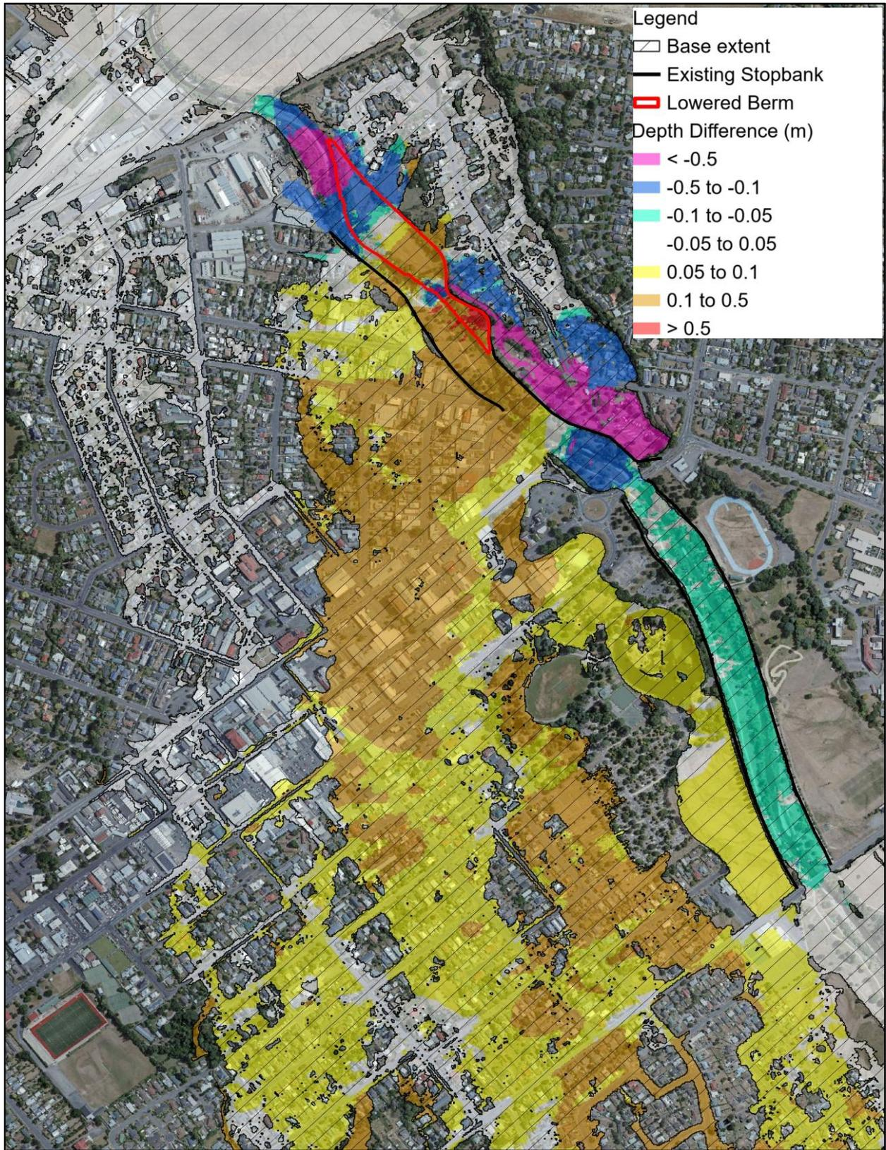
Figure 3-9: 1% AEP flow depth difference layer
