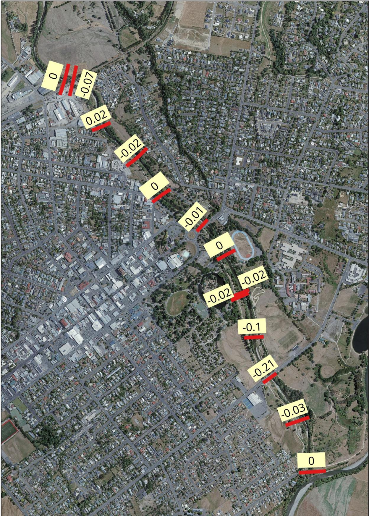
Figure 2-2: Map of the difference (in unit m) between calibrated 2D Waipoua model water levels and the surveyed debris levels from the Oct 1998 flood event
