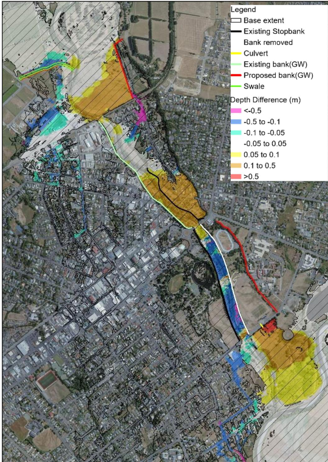
Figure 3-48: Combined Option 2 depth difference map (with bund at Akura).
