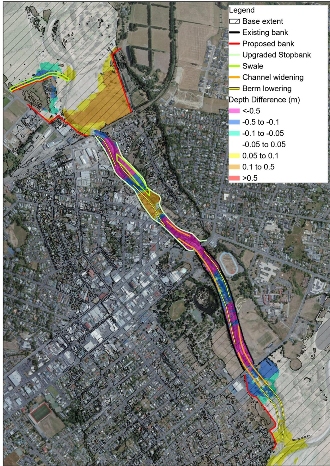
Figure 3-84: Final Iteration Option 2 depth difference map
