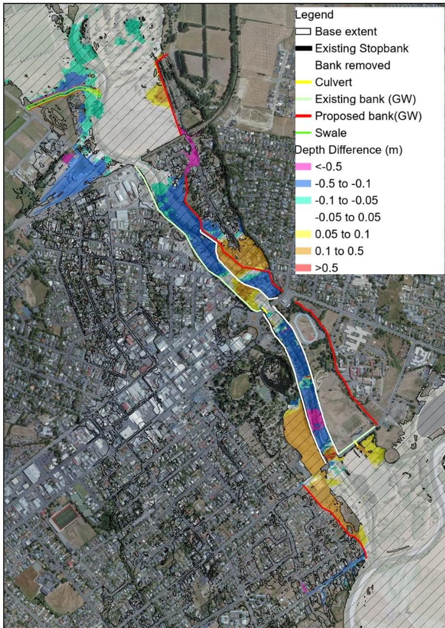
Figure 3-54: Combined Option 5 depth difference map (with bund at Akura).
