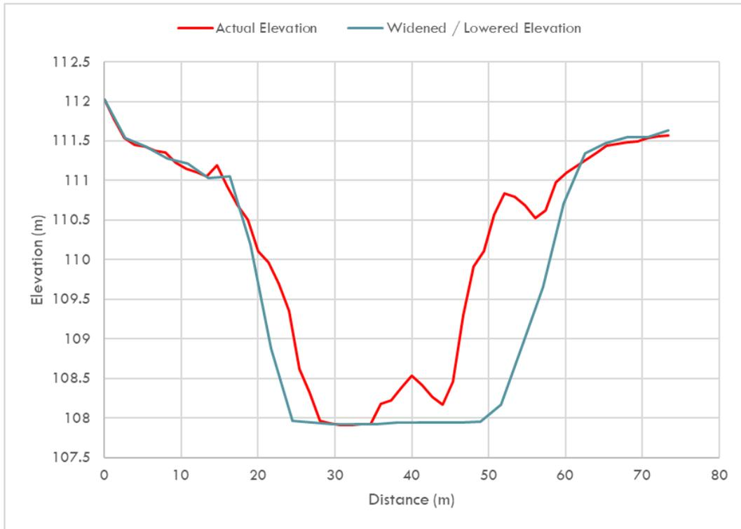
Figure 3-68: Example of channel widening immediately downstream from Colombo Rd Bridge.
