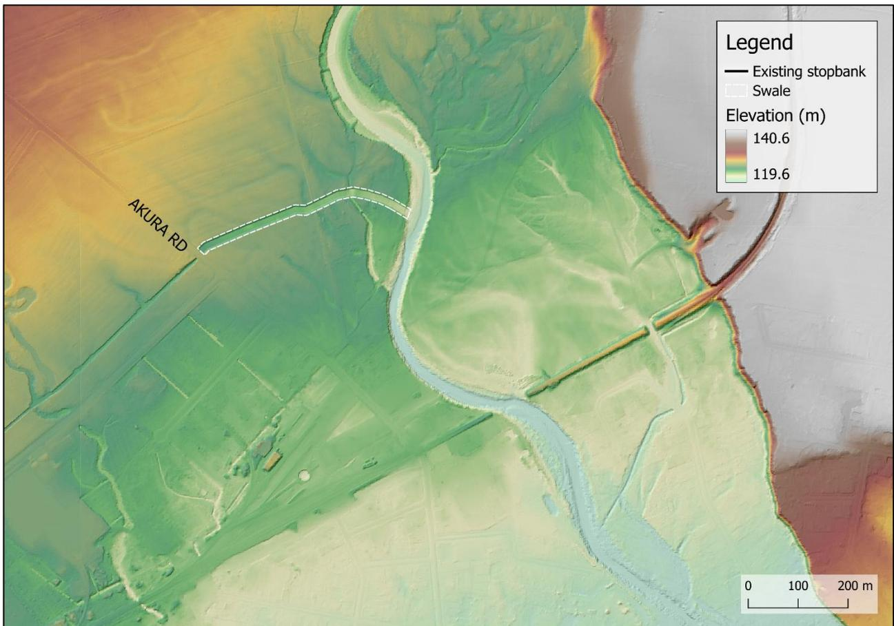
**Figure 3-6: Option 2 with swale at Akura**
