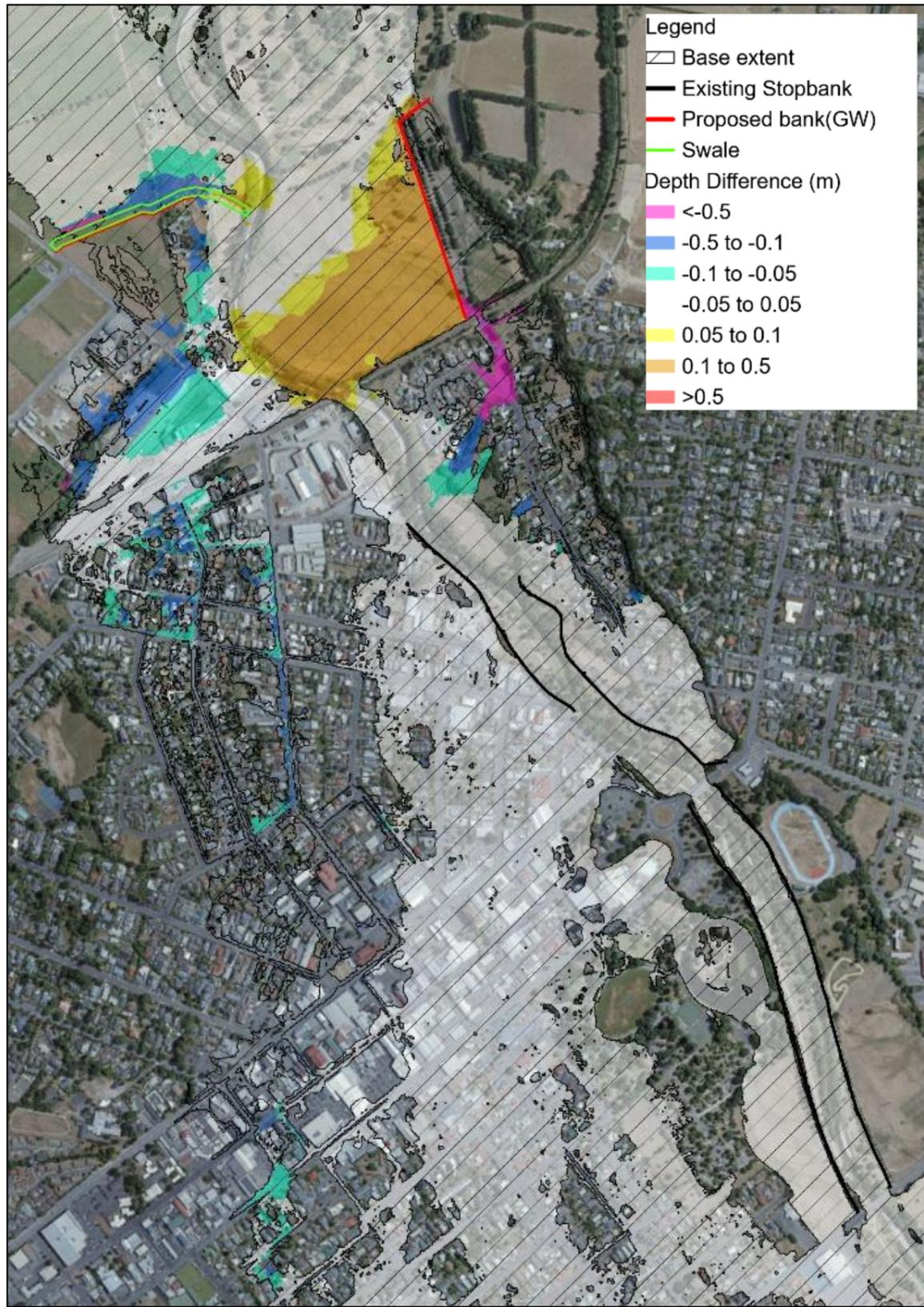
Figure 3-45: Combined Option 1A depth difference map (with bund at Akura Rd swale).
