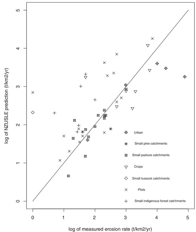
**Figure 4.** Plot of NZUSLE predictions versus measured rates of surficial erosion spread throughout New Zealand. The value of  $R^2$  is 0.60.
