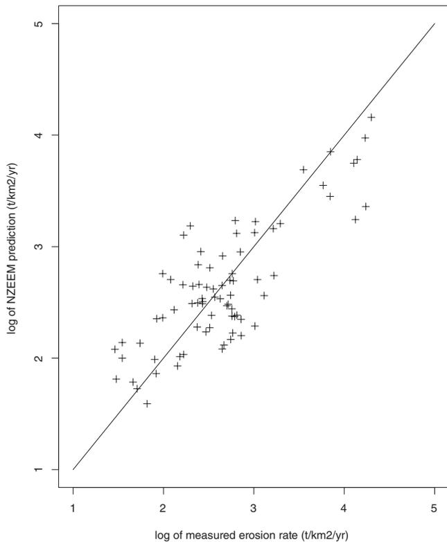
**Figure 3.** Plot of NZEEM<sup>®</sup> predictions versus measured specific sediment discharge for 80 long-term measurement sites spread throughout New Zealand. The value of  $R^2$  is 0.65.
